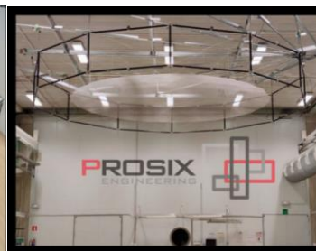
Figure 2-47 Extendable/Deployable Truss for Membrane Single Modules SBSP
