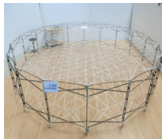
Figure 2-47 Extendable/Deployable Truss for Membrane Single Modules SBSP
