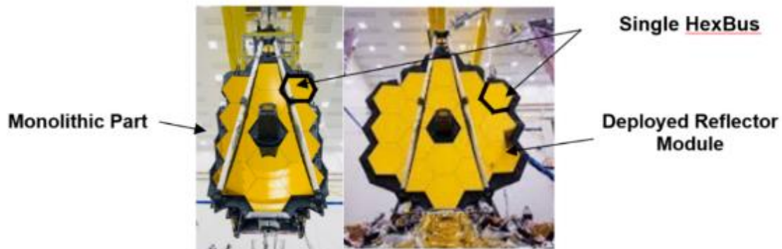
Figure 2-30 Concept for Reflector Module in-flight (folded) & in-orbit (deployed) Configuration (courtesy of NASA)
