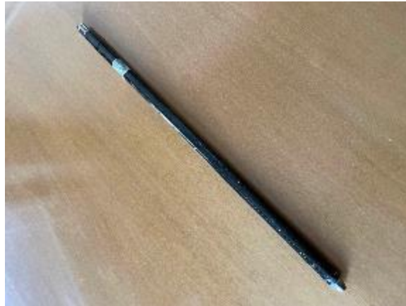
Figure 2-33 Truss Strut for the “Ring Structure”
