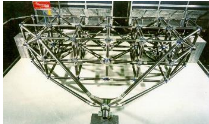
Figure 2-37 Truss Structure Example
