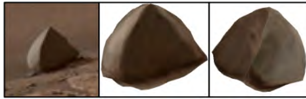
Figure 4: On the left, identified rock with Yolov5 from Perseverance rover Navcam. On the middle and right images, reconstructed 3D model from two points of views using Unicorn GAN.
