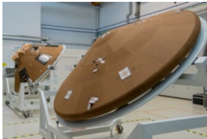
Figure 3-6: Aeroshell Configuration Overview (heritage from ExoMars 2016)
