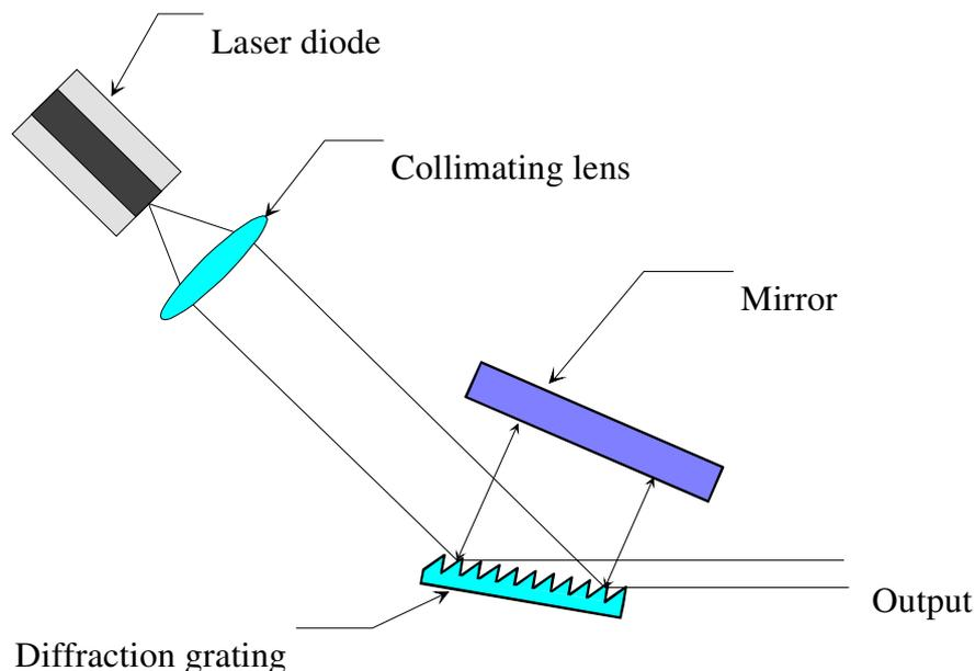
**Fig. 7.1.4-2 Scheme of the Littman-Metcalf cavity.**
