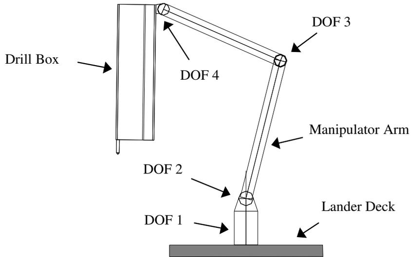
**Fig.5-1 Drill Box and Manipulator Arm (DeeDri in '03/'05 project)**
