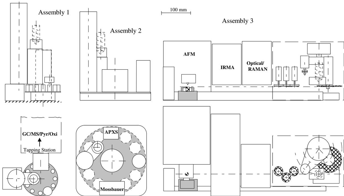
**Fig.6-1 SPHS (Three Independent Assemblies)**
