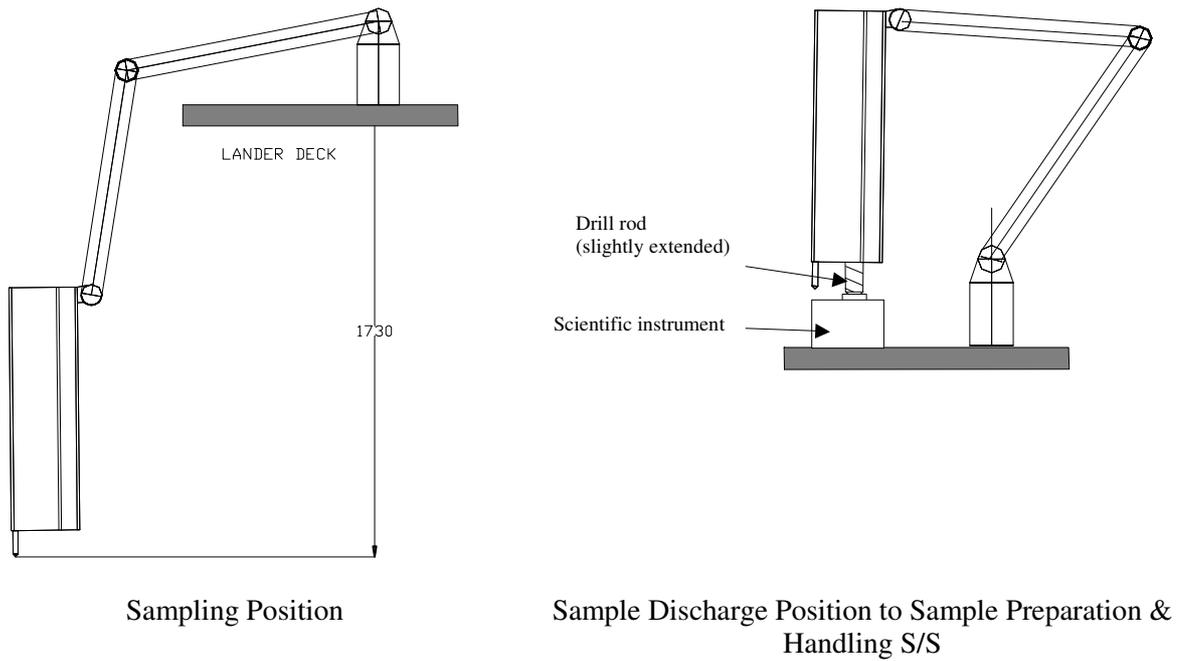
**Fig.5-2 Drill Box and Manipulator Arm Operations (drilling and sample discharge)**
