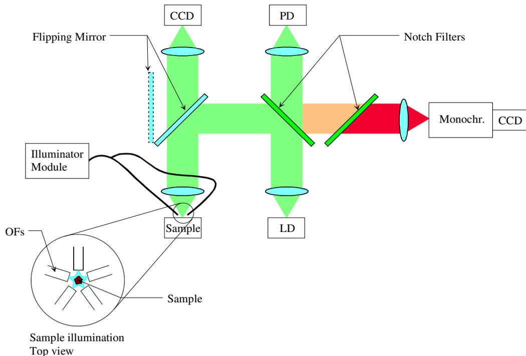
**Fig.7.1.4-1. Principle block scheme of the proposed instrument.**
