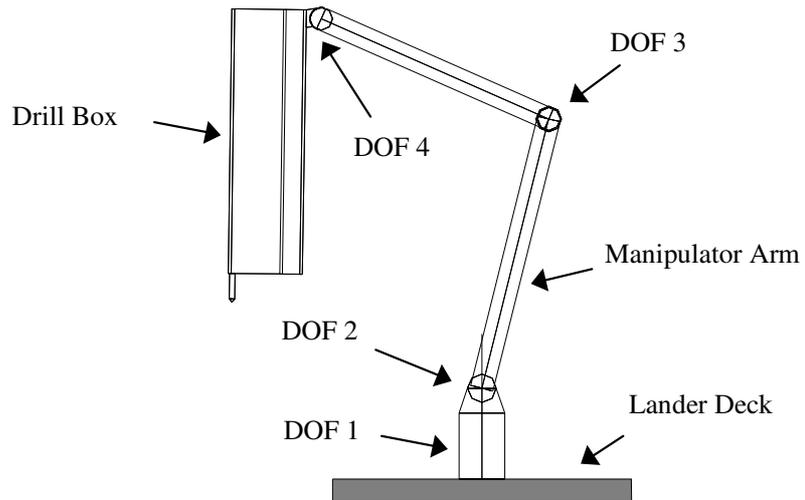
**Fig.4.6-3 Drill Box and Manipulator Arm (4 DOF, 1.7 m deck height capability) on Lander**
