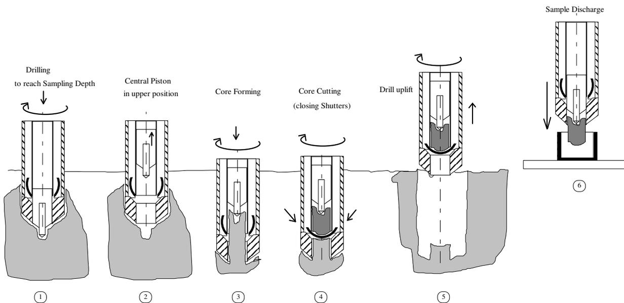
**Fig.5-4 Sample Acquisition Procedure**
