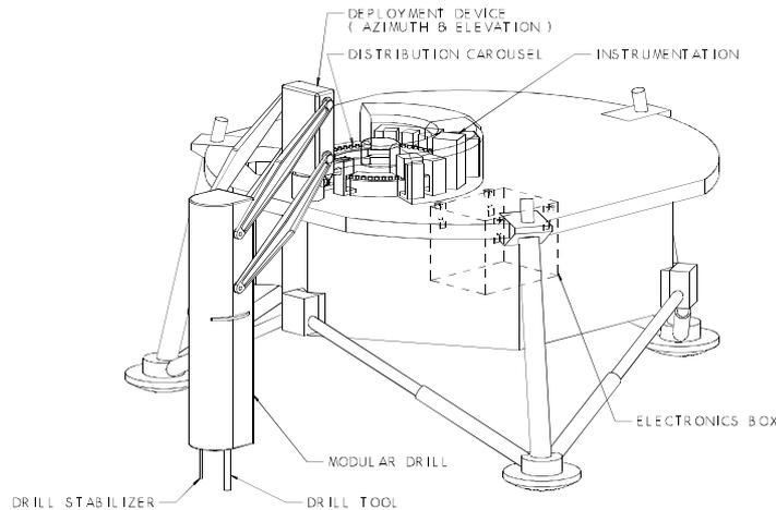
**Fig.4.6-1 EMF on Lander, Drill Operation (pictorial view)**
