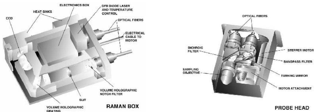
**Fig.7.1.2-1 Athena Raman Spectrometer**
