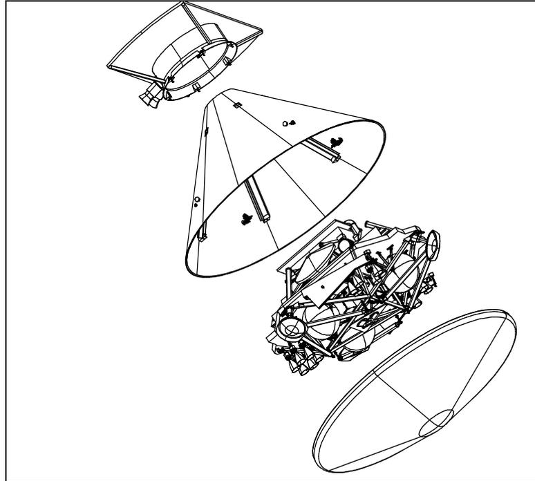
**Fig.2-3 Exploded View of lander, Cruise Stage & Aeroshell**
