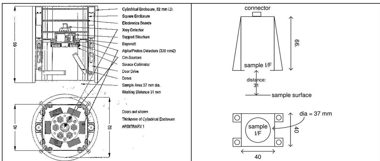
Fig. 7.2.1-1 Sensor Head Design
