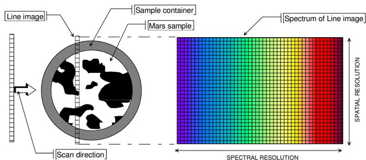
Fig.7.1.3-2 Scheme of image cube acquisition
