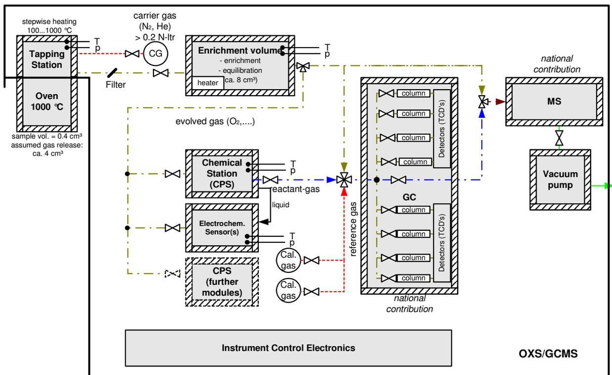
Fig.7.2.4-1 Schematic Overview of the combined OXS/GCMS Instrument
