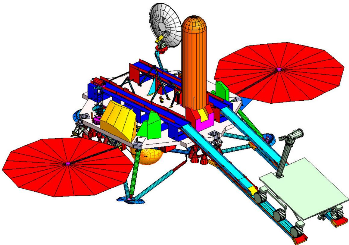
**Fig.2-1 Lander with Rover & MAV deployed and Additional Payload areas depicted,
