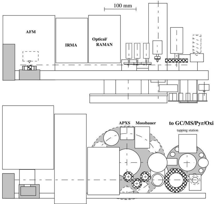
**Fig.6-2 SPHS (Integrated Assemblies)**
