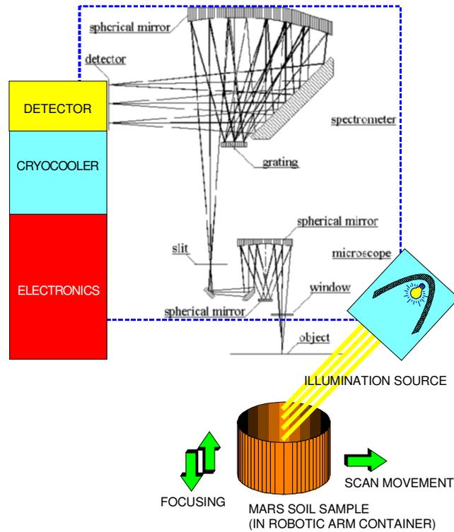
Fig.7.1.3-1 Schematic concept of IRMA instrument (Optics design by Dr A. Romoli)
