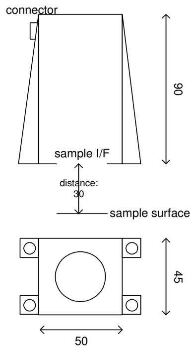
**Fig.7.2.2-1 Possible configuration of the Mössbauer spectrometer sensor head on EMF**
