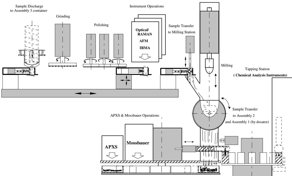
**Fig.6-3 SPHS (Integrated Assemblies) Sample Processing Flow**
