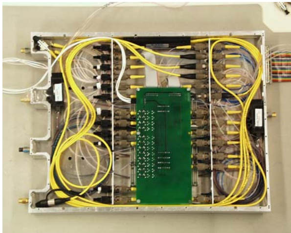
Figure 9 Switched Fibre beamformer prototype
