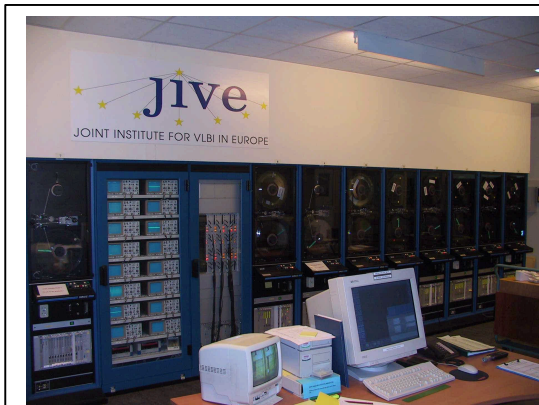
Fig. 4-9. EVN MK4 Correlator at JIVE, a dedicated 60 TeraOps supercomputer
