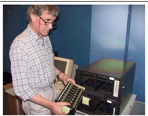
Fig. 4-10. Mk5 disk based VLBI recorder/playback unit and a removable 1.6 TeraByte disk pack
