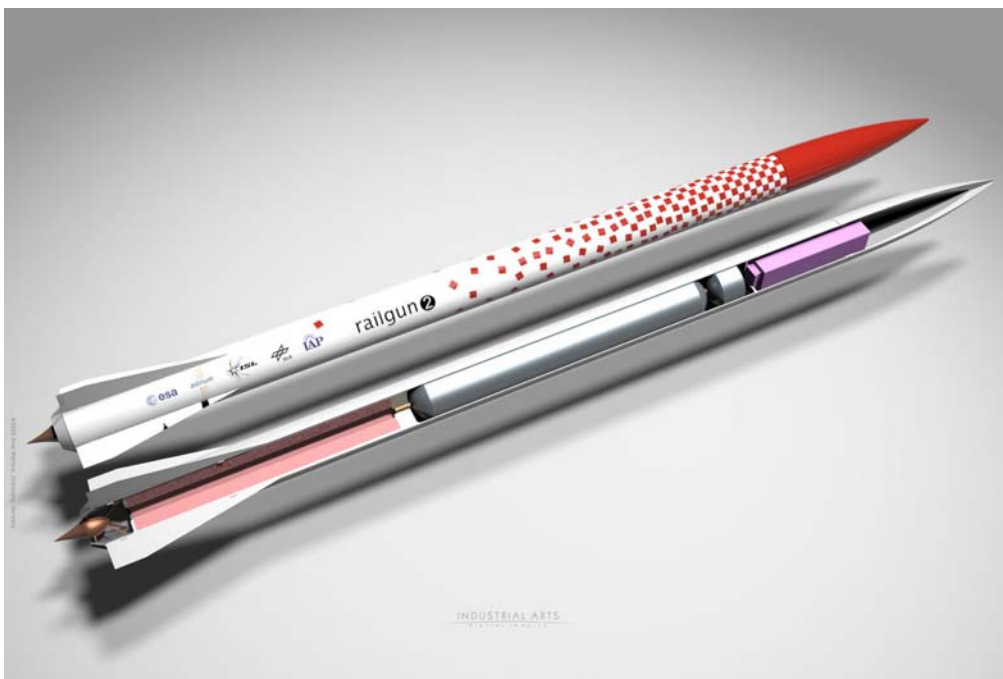
Figure 28 Propelled orbital payloads projectile layout – optimised configuration
