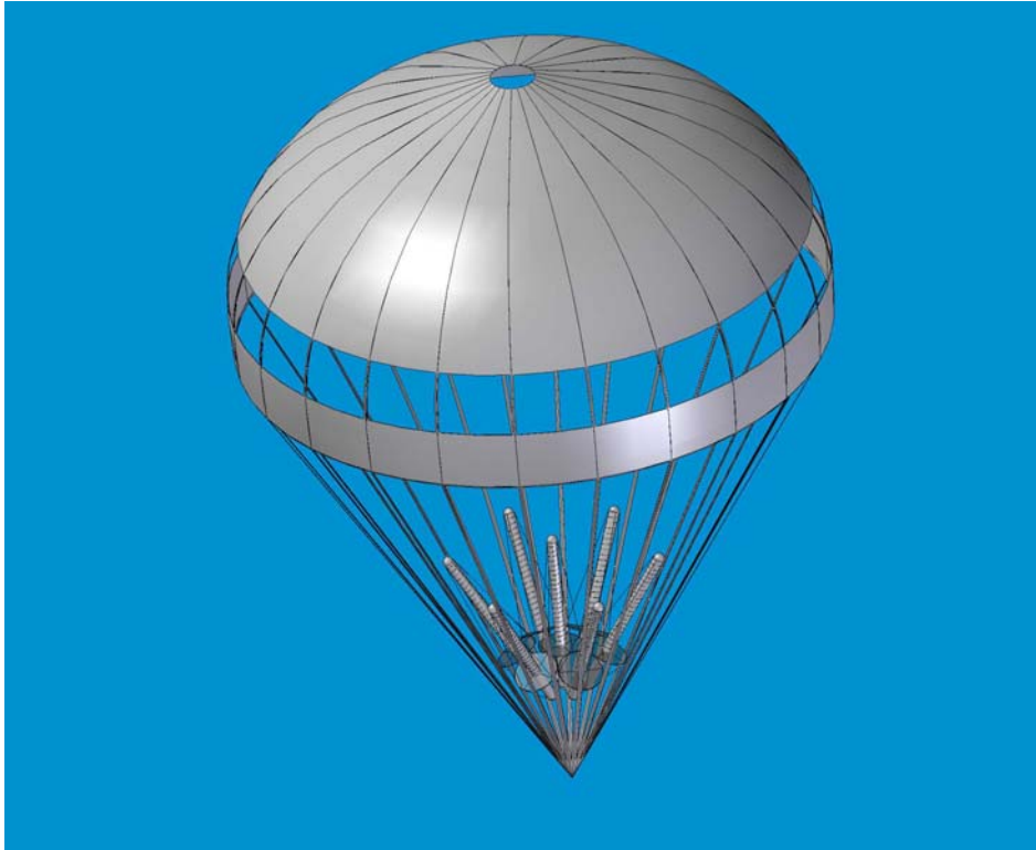
Figure 5-1 Antenna concept design within parachute
