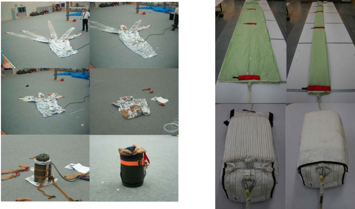
Figure 5-2 Inflatable and Parachute packing sequence
