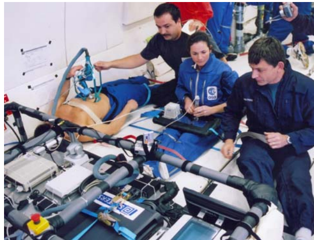
Figure 2: test of the robotic tele-echography system in weightlessness (Picture credit: ESA)
