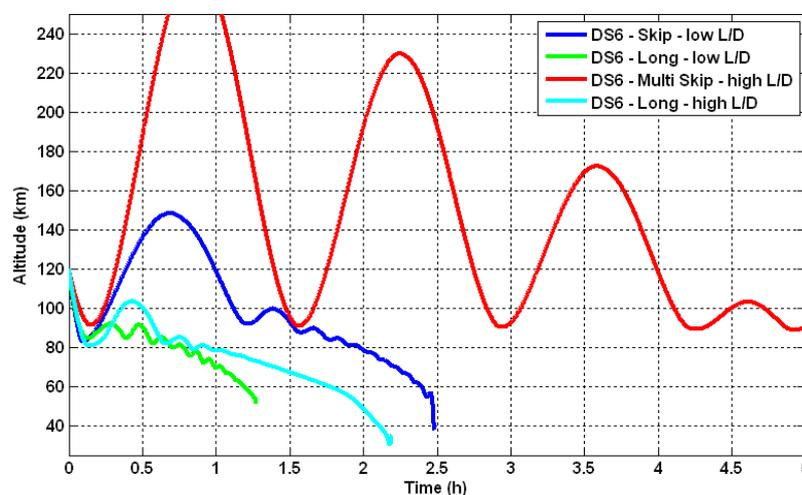
*Fig. 5-13. Optimum entry trajectories performing different entry techniques: long entry, skip entry and multi-skip.*
