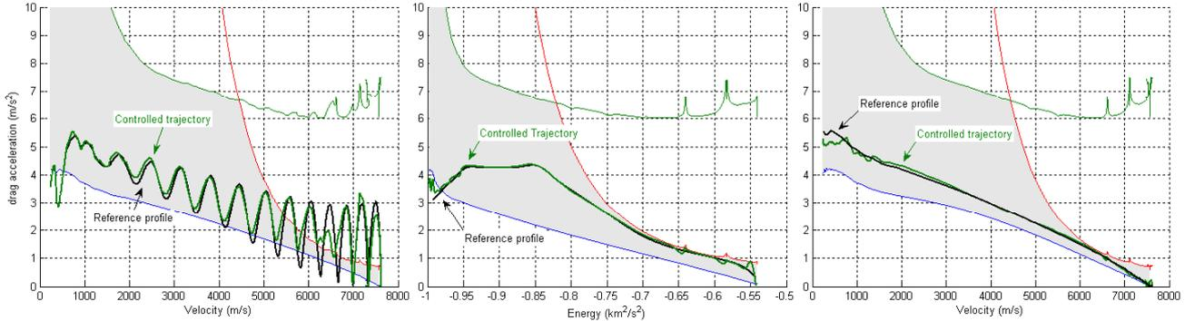
**Fig. 5-16. Reference and controlled drag profiles for the study case 1 (left), 2 (center), and 3 (right).**
