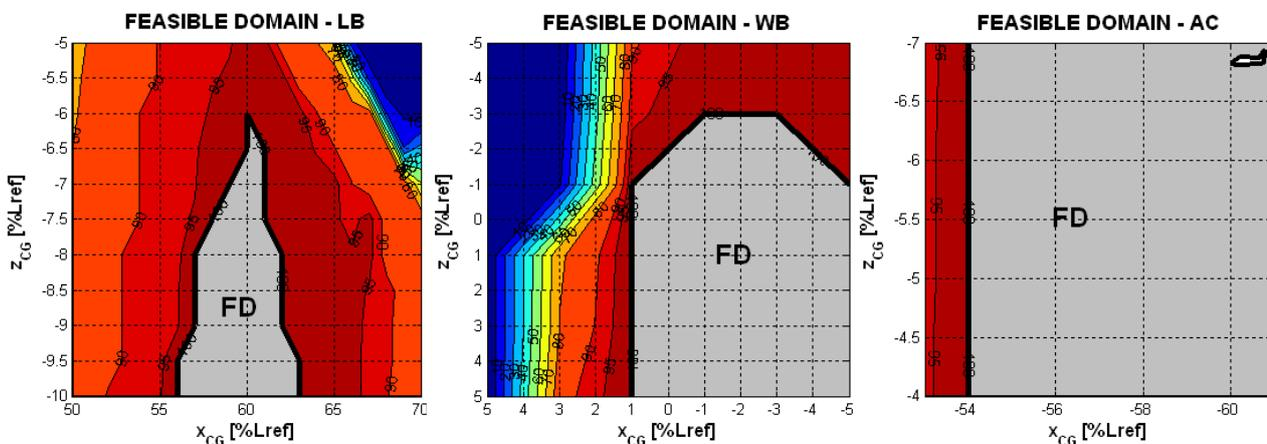
*Fig. 5-10. Feasible Domain (FD) for Lifting Body (LB), Winged Body (WB) and Advanced Concept (AC)*
