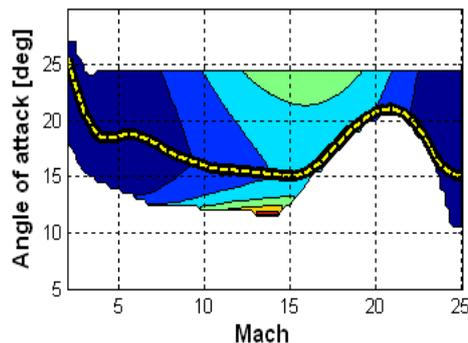
*Fig. 5-12. Optimum trim for the optimum COG for the Advanced Concept*
