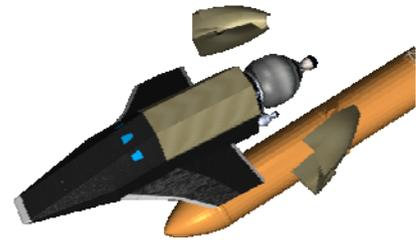
*Fig. 5-4. The DS architecture with cargo bay doors open and solar arrays deployed*
