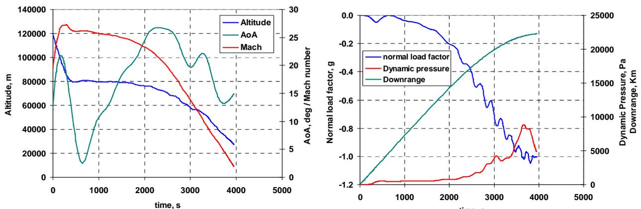
*Fig. 5-23. USV-X concept expected mission profile.*
