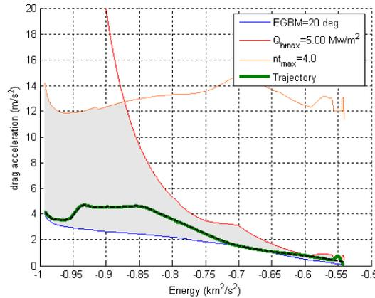
*Fig. 5-18. Reference and controlled drag profile, reference scenario*
