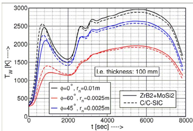
**Fig. 5-8. Effect of materials and swept angles on adiabatic wall temperatures**
