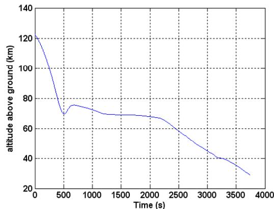
*Fig. 5-19. Long entry altitude profile, reference scenario*
