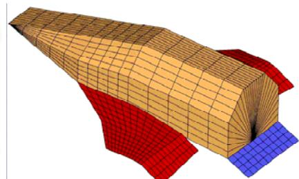
*Fig. 5-3. advanced concept (sharp leading edge)*
