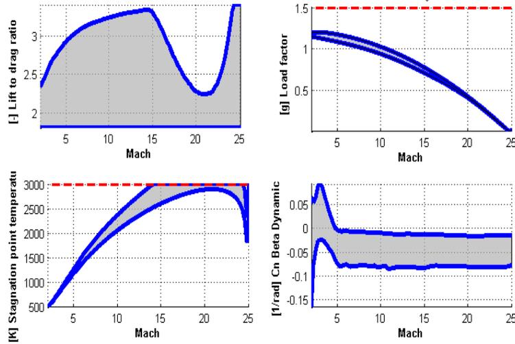
*Fig. 5-11. Envelope of performances for the Advanced Concept (Grey region: Corridor, Red: Constraints)*
