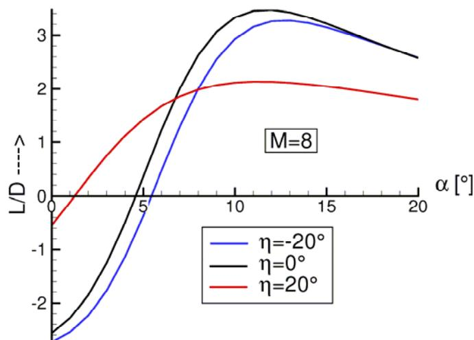
*Fig. 5-7. hypersonic Lift-to-Drag ratio of the DS6 vehicle*
