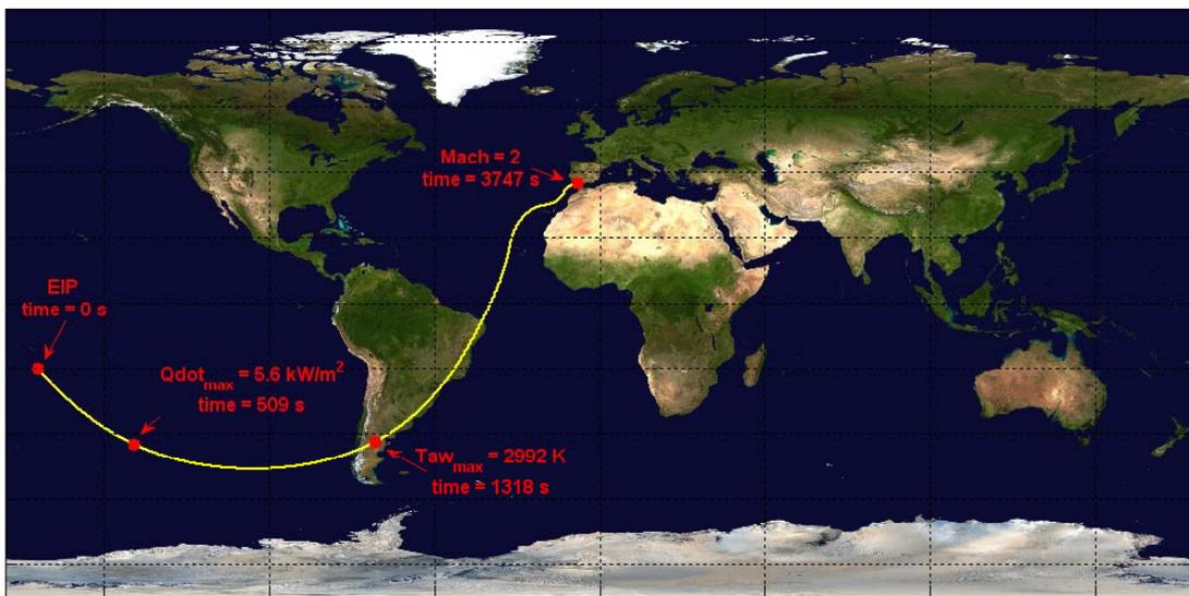
*Fig. 5-20. Ground track and re-entry events, reference scenario*
