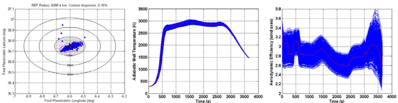
*Fig. 5-21. Performance assessment results: accuracy at Mach 2 (left), adiabatic wall temperature dispersion (centre), and aerodynamic efficiency dispersion (right).*
