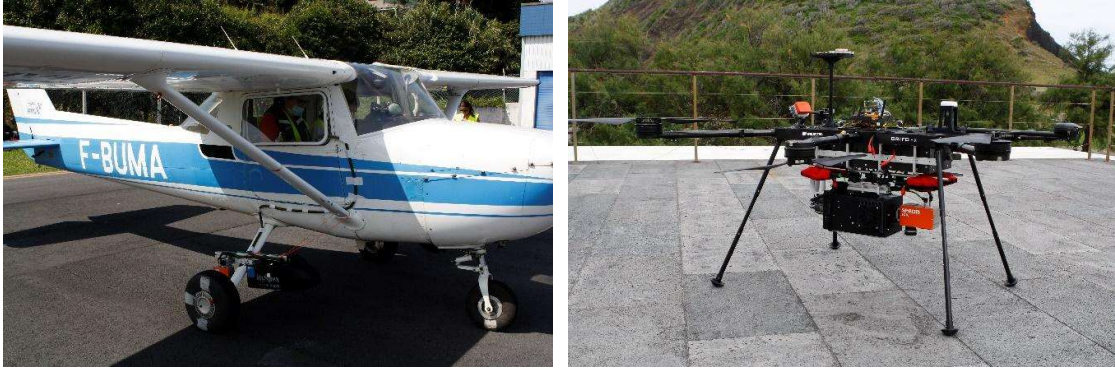
Figure 7 - Manned Piloted Aircraft with the hyperspectral cameras on the landing gear, and Grifo-X UAV equipped with the hyperspectral cameras on the landing platform
