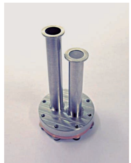
Photograph of the breadboard during assembly. The cold finger is not yet wrapped in Mylar nor placed in the vacuum vessel.
