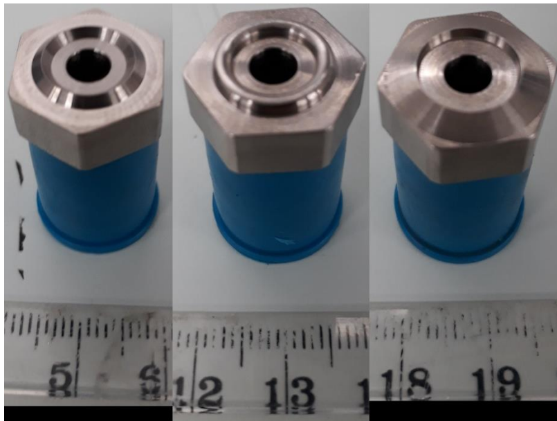
Figure 1: Machined knife-edge attachments. L-R: 90°, VCR-Type, CF-type
