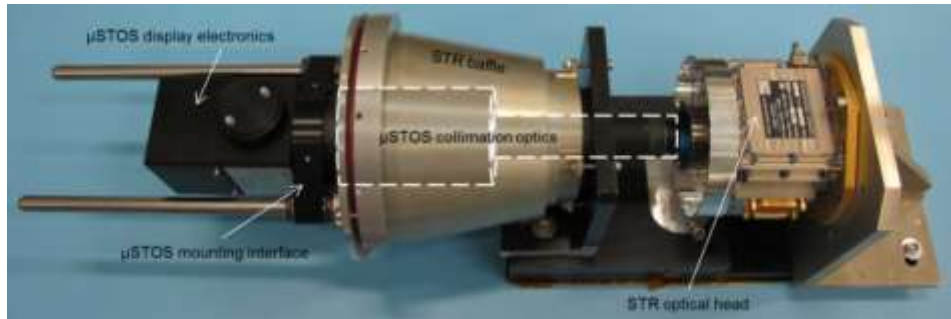
Figure 2: A description of the STOS opto-mechanical assembly (on a Sodern SED36 sensor)
