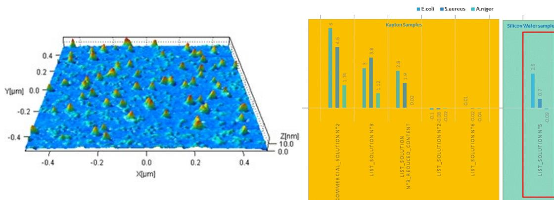
Figure 7. (left) AFM images of nanopatterned ultrathin ZnO films; (right) Inside the red rectangle, antimicrobial Activity, R (logarithm reduction of the number of surviving micro-organisms in cells/cm<sup>2</sup>) of antimicrobial nanopatterned ZnO coatings deposited on silicon wafer for *E. coli* (left), *S. aureus* (center) and *A. niger* (right)
