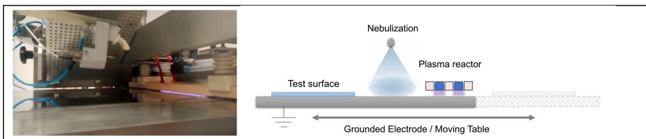
**Figure 1. Atmospheric-pressure plasma polymerization setup developed at LIST for large area surfaces and the schematic representation of its fundamental parts**
