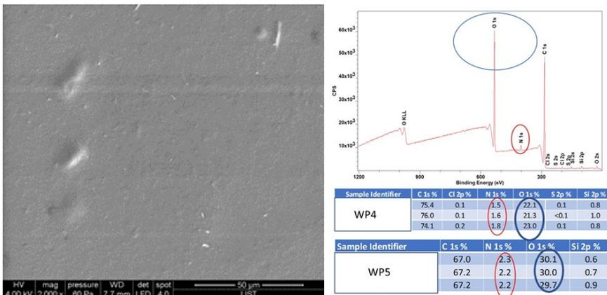
Figure 10. (left) SEM images of up-scaled PVA-based coatings embedding lignin nanoparticles; (right) XPS analyses on PVA-based coatings embedding lignin nanoparticles
