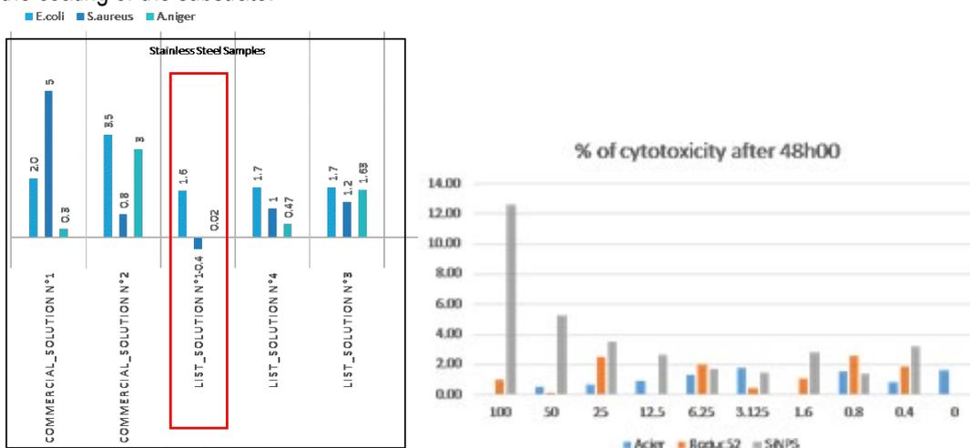
Figure 2. (left) Inside the red rectangle, antimicrobial Activity, R (logarithm reduction of the number of surviving microorganisms in cells/cm<sup>2</sup>) of antimicrobial HMDSO-based hydrophobic coatings deposited on stainless steel for *E. coli* (left), *S. aureus* (center) and *A. niger* (right); (right) Cytotoxicity (%) on human skin keratinocytes cells with the LDH assay on HMDSO-based hydrophobic plasma coatings (in orange).
