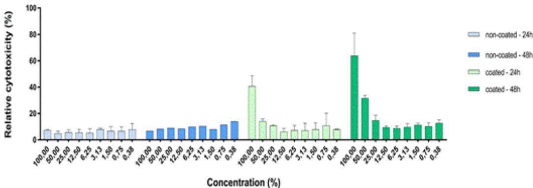
**Figure 5. Cytotoxicity (%) on human skin keratinocytes cells with the LDH assay on non-coated stainless steel (blue) and on PVA-based coatings embedding lignin nanoparticles (0.15 w.%) (green)**
