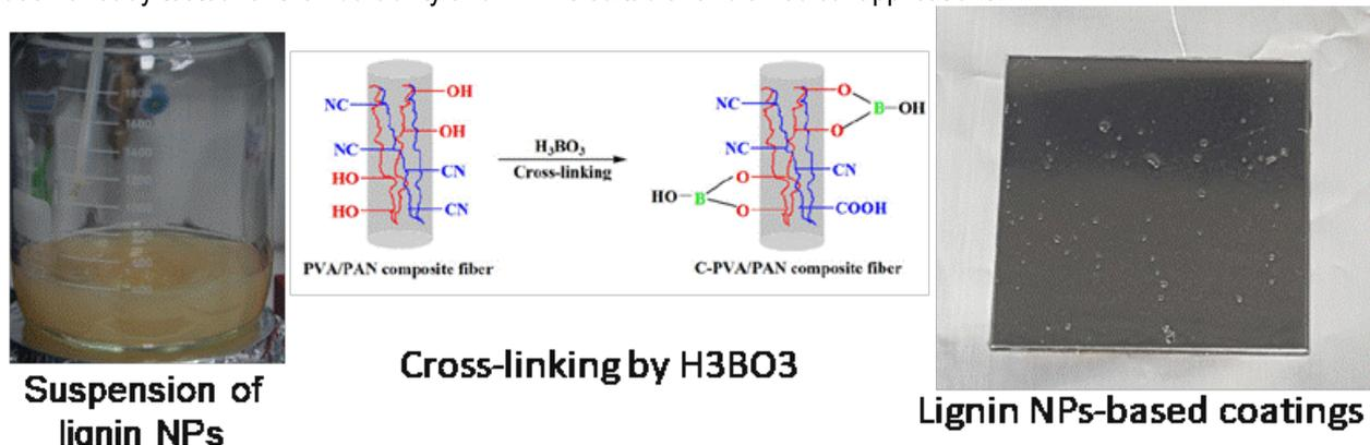
Figure 3. Fabrication of PVA-based coatings embedding lignin nanoparticles
