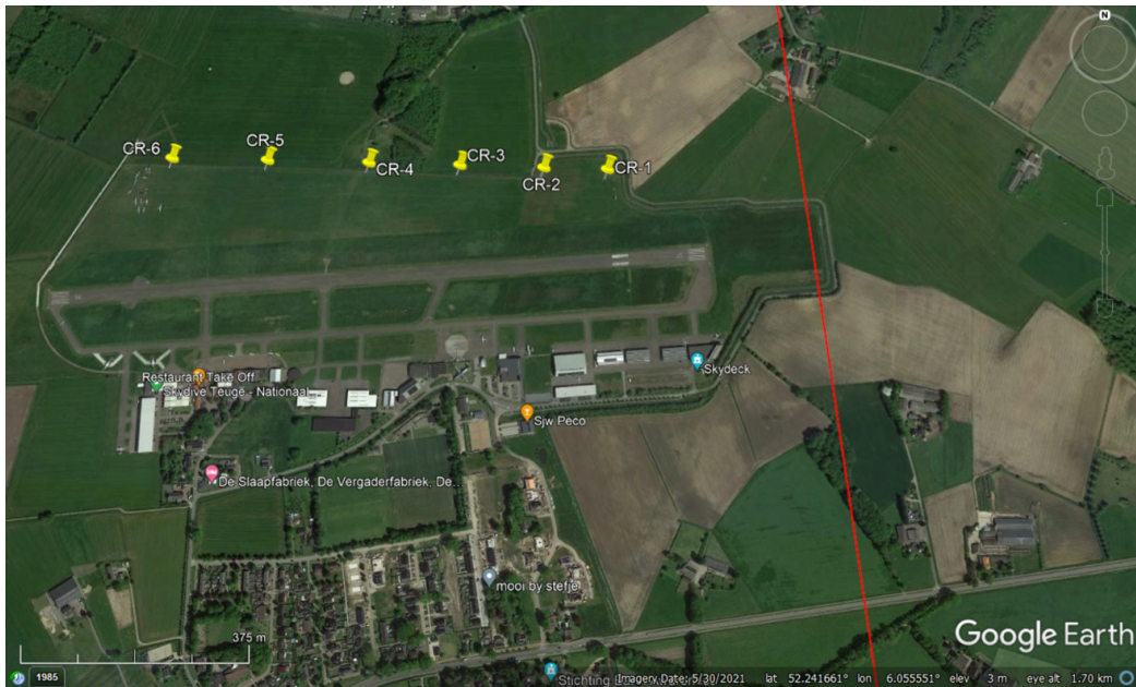
Figure 6: Position of the corner reflectors (yellow pins) and the track of the flight (red line)
