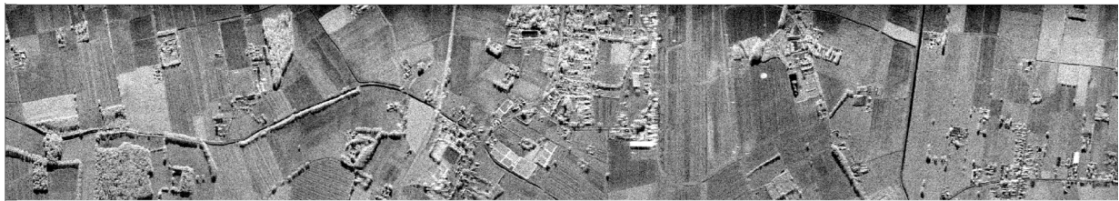
Figure 4: SAR image generated by the KaSAR Processor from data acquired by KaSAR
