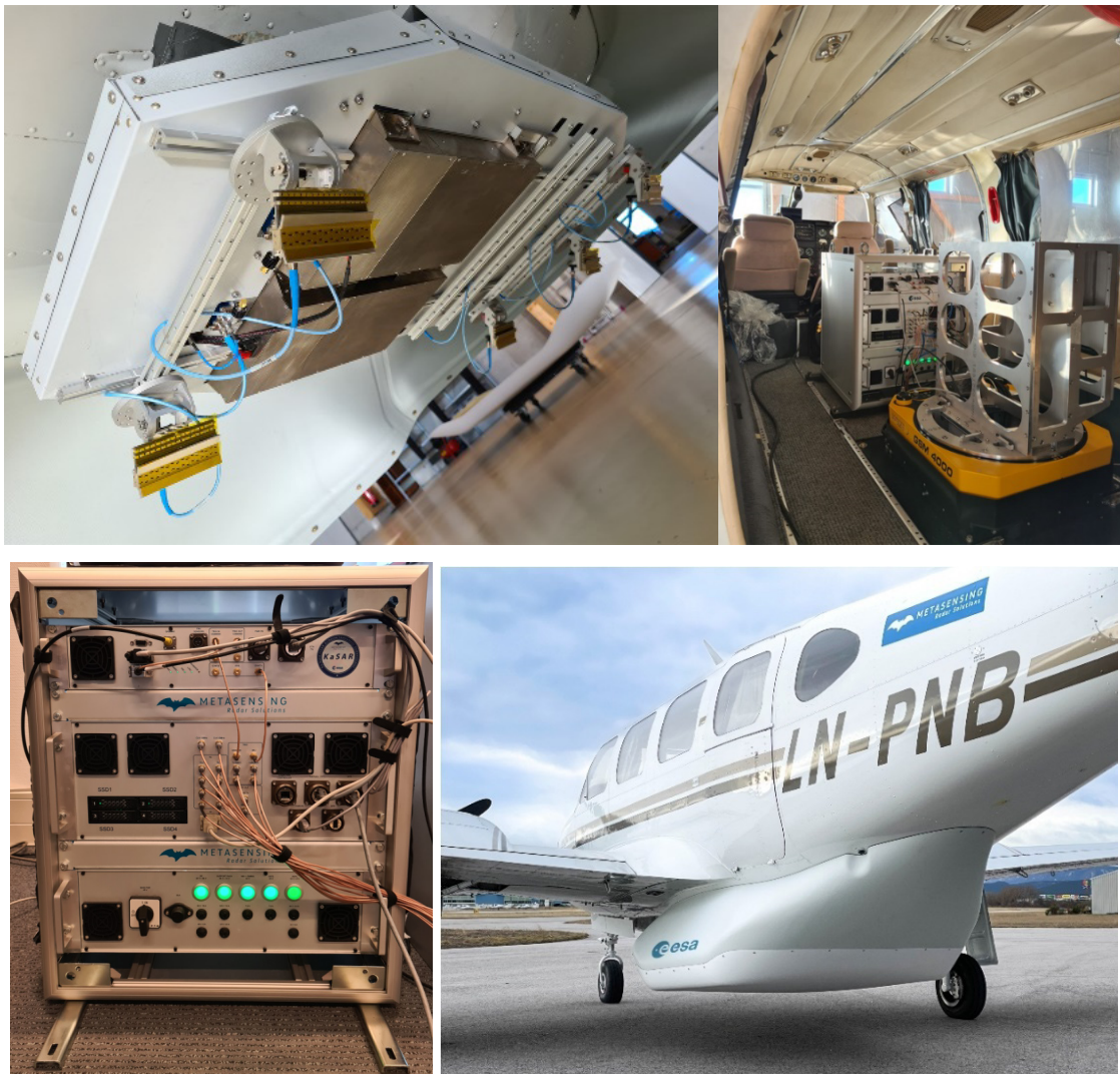
Figure 3: KaSAR instrument installed on Piper PA031
