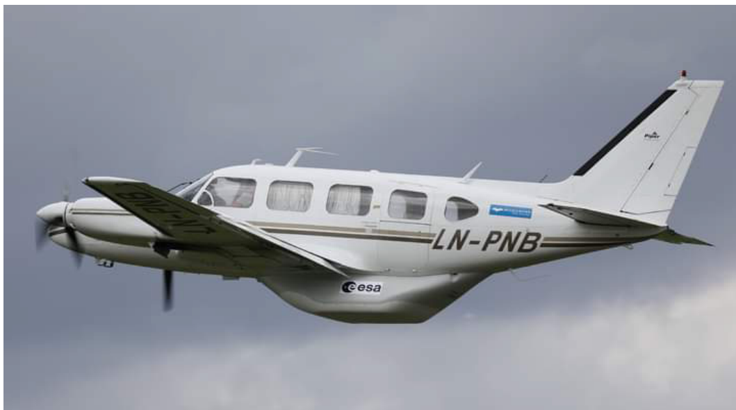
Figure 1: MetaSensing's Piper PA-31 with the belly pod hosting the KaSAR instrument
