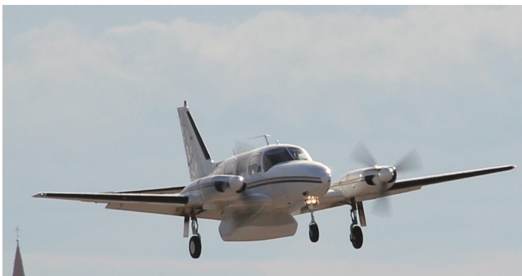
Figure 5: Piper PA31 aircraft modified with the belly pod for KaSAR
