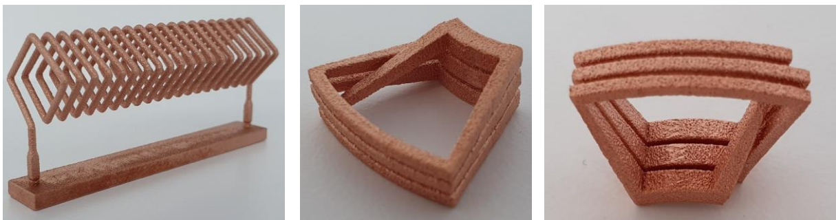
Figure 4-1: Benchmark geometries produced by L-PBF with green laser source
