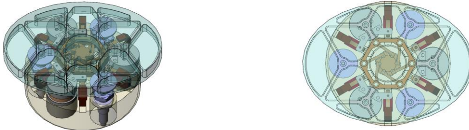
Figure 3-2: ISABELA FSM concept baseline, with elliptical mirror, isometric view (left), upper view (right)
