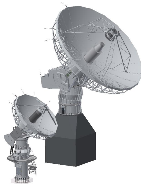
Figure 1-1: S/X-band 6.8m and S/K-band 14m 3-axes full motion antennas
