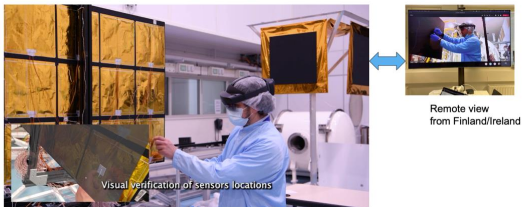
Figure 4. The set-up for the remote user test of the MR system. Left: Actual system installation in ESA-ESTEC. Right: Video and audio feed for observation teams in Finland and Ireland
