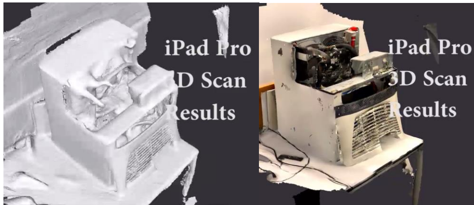
Figure 6-1 iPad Pro 3D Scan Results (Left: Untextured, Right: with Texture)
