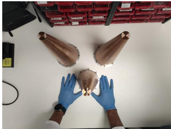
Figure 3. HFWF CLSA feed – Assembly of breadboards into laboratory.
