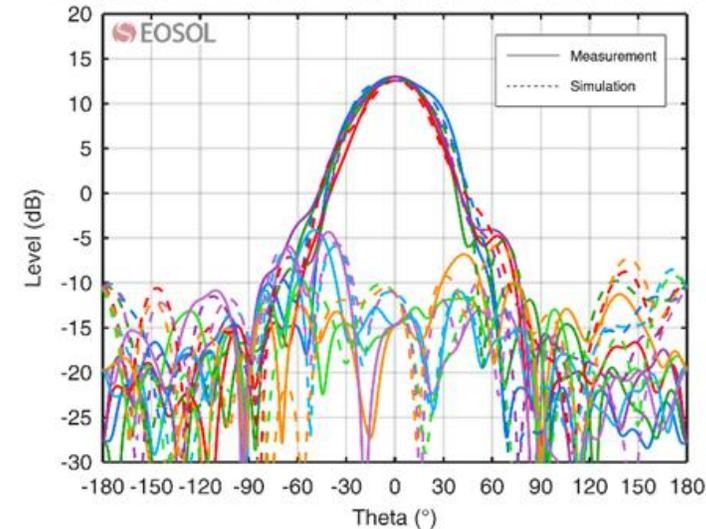
Embedded HFWF-Sub-Array SN106 Rad Pattern at 1.5 GHz
