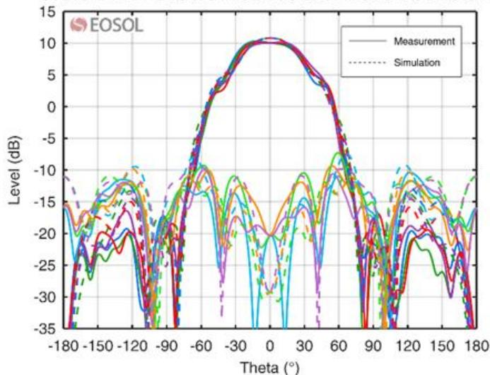
CRYO HF WF-CLSA SN103 Radiation Pattern at 2.0 GHz
