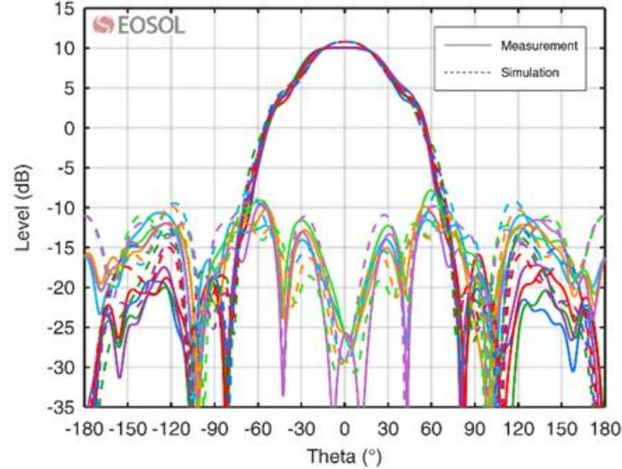
CRYO HF WF-CLSA SN104 Radiation Pattern at 2.0 GHz
