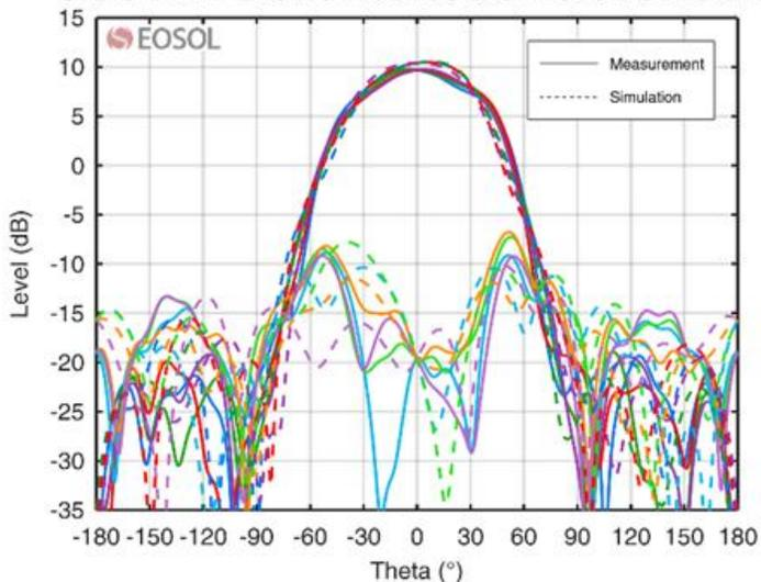
CRYO HF WF-CLSA SN103 Radiation Pattern at 1.9 GHz
