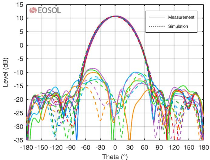
CRYO HF WF-CLSA SN103 Radiation Pattern at 1.0 GHz
