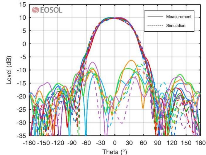
CRYO HF WF-CLSA SN103 Radiation Pattern at 1.5 GHz
