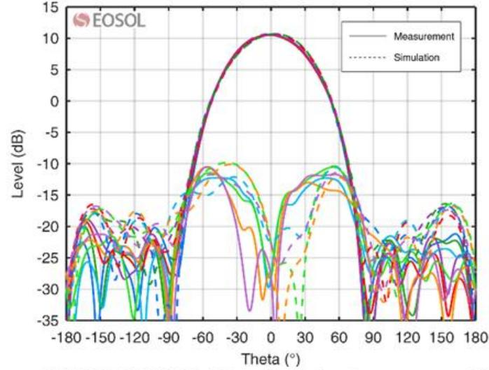
CRYO HF WF-CLSA SN105 Radiation Pattern at 1.4 GHz
