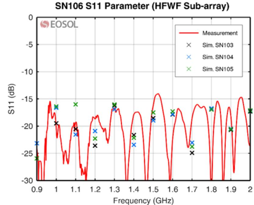
The measured **S11 parameter** results are under -15 dB in the complete frequency band except at 1.52 GHz where it increases to -14 dB.
