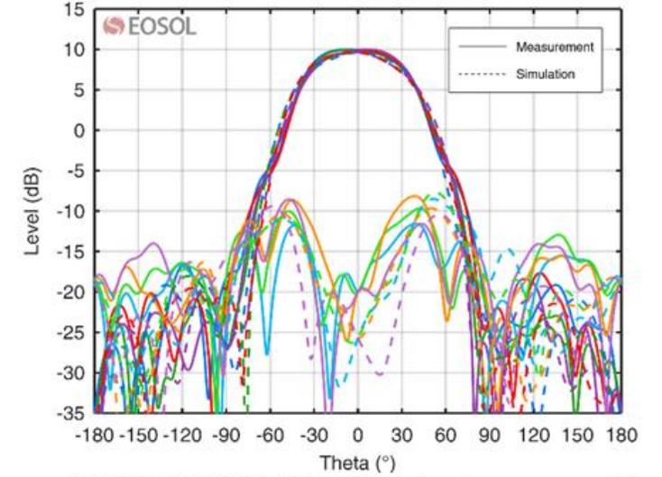
CRYO HF WF-CLSA SN104 Radiation Pattern at 1.5 GHz
