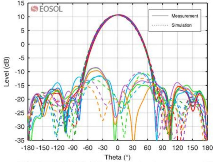
CRYO HF WF-CLSA SN105 Radiation Pattern at 1.0 GHz
