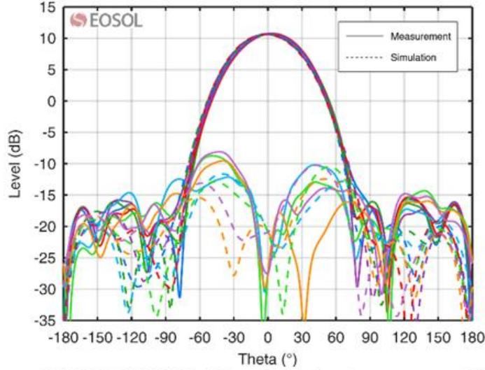
CRYO HF WF-CLSA SN104 Radiation Pattern at 1.0 GHz
