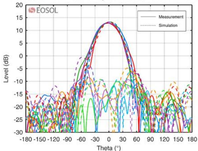
Embedded HFWF-Sub-Array SN106 Rad Pattern at 1.9 GHz
