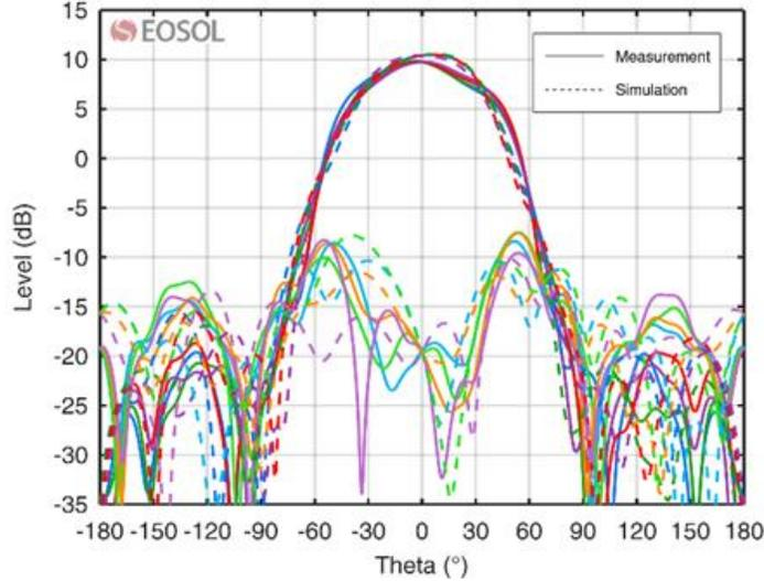
CRYO HF WF-CLSA SN105 Radiation Pattern at 1.9 GHz
