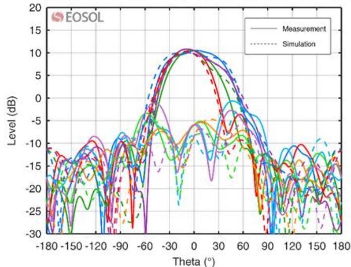
Embedded HFWF-Sub-Array SN106 Rad Pattern at 1.4 GHz
