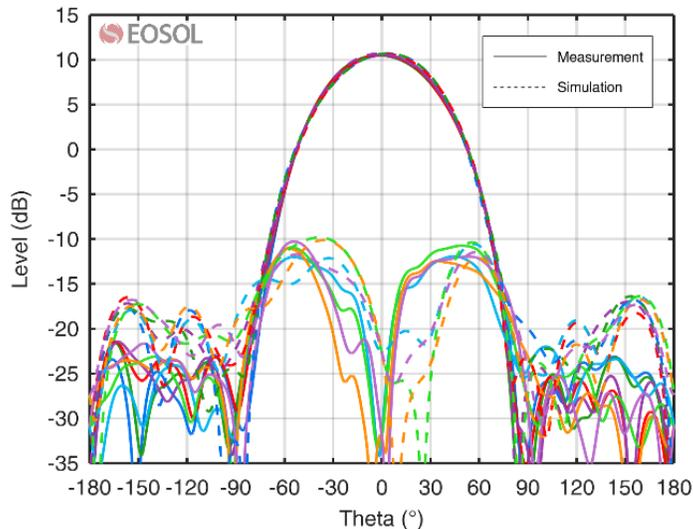
CRYO HF WF-CLSA SN103 Radiation Pattern at 1.4 GHz
