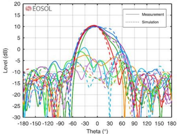
Embedded HFWF-Sub-Array SN106 Rad Pattern at 1.0 GHz
