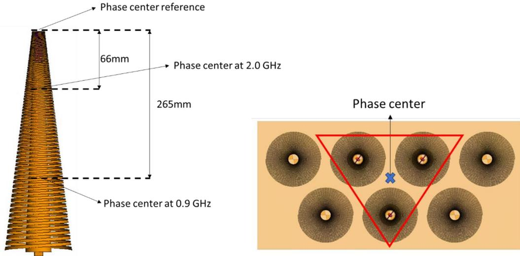
Embedded sub-array phase center location reference figures
