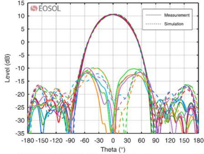
CRYO HF WF-CLSA SN104 Radiation Pattern at 1.4 GHz
