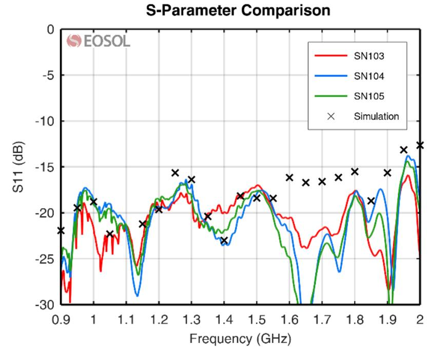
The measured **S11 parameter** results are typically under -15 dB in the complete frequency band.
