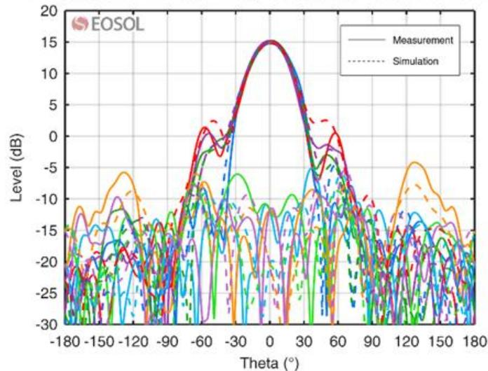
Embedded HFWF-Sub-Array SN106 Rad Pattern at 2.0 GHz
