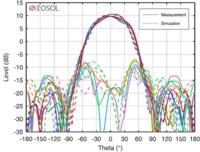
CRYO HF WF-CLSA SN104 Radiation Pattern at 1.9 GHz
