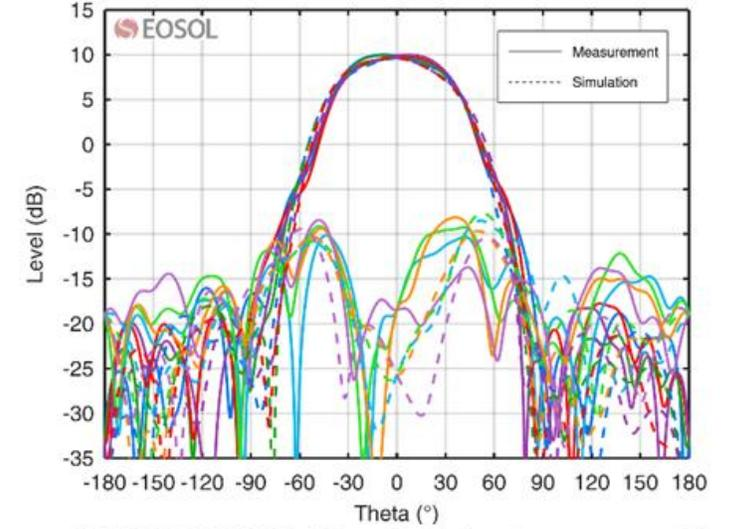
CRYO HF WF-CLSA SN105 Radiation Pattern at 1.5 GHz
