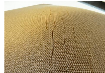
Antenna reflector shape Sheet thickness: 19 mm
