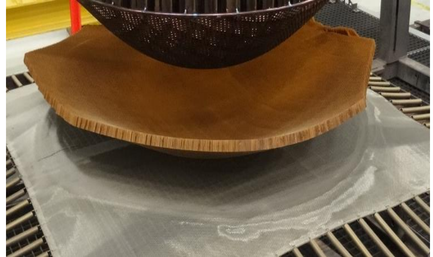
Antenna reflector shape Sheet thickness: 19 mm
