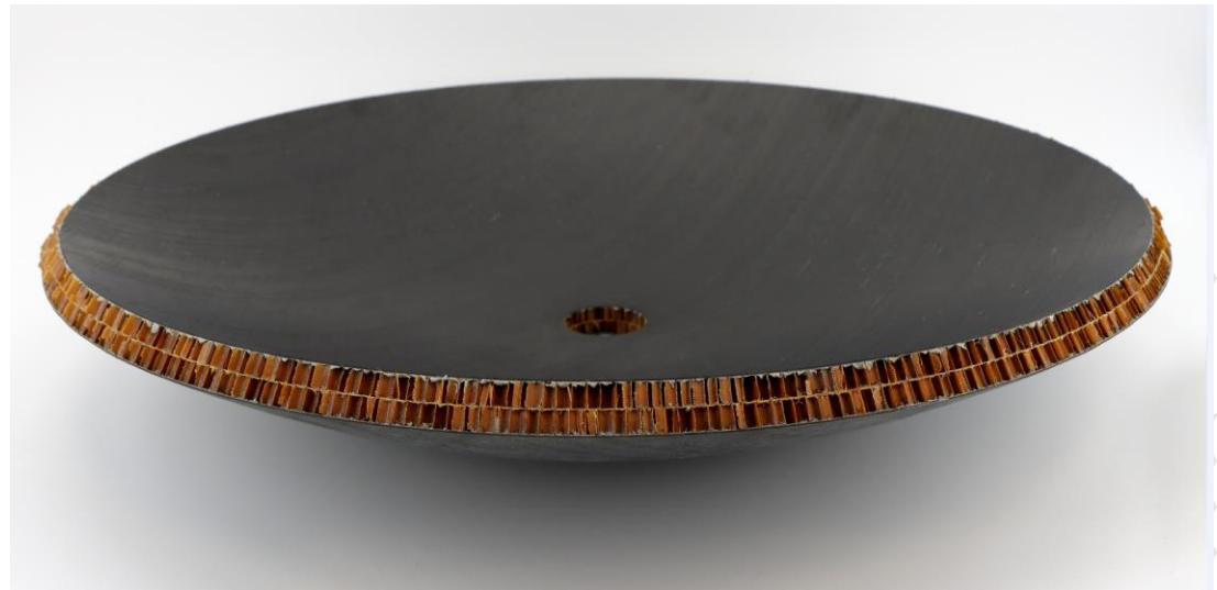
Trimmed segment on the lay up tool
