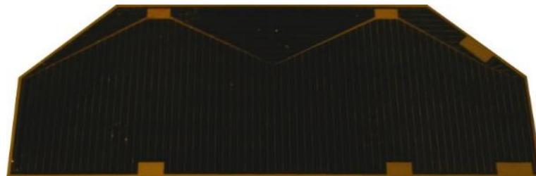
Figure 3-6: Example of a 20 cm<sup>2</sup> ultra-thin IMM-4J space solar cell.
