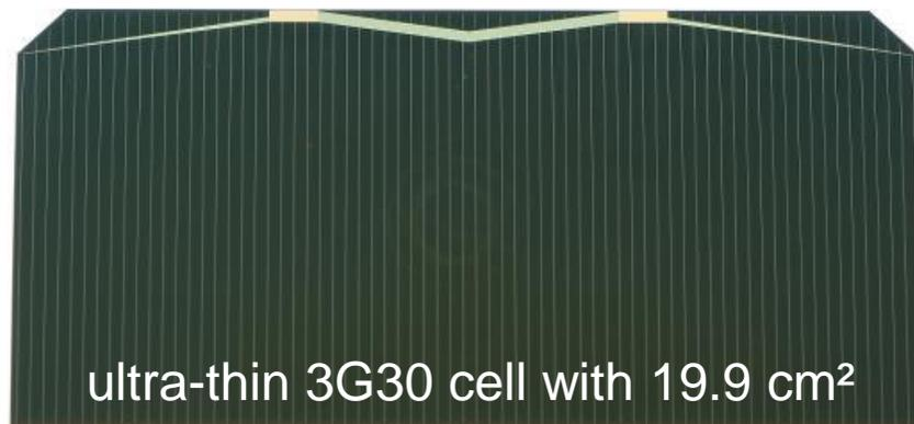
$$\eta_{\text{avg}} = \mathbf{29.0\%} \text{ (AM0, 1367 W/m}^2\text{, 25}^\circ\text{C)}$$
