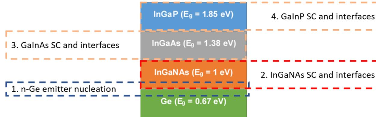
Fig. 2: Basic principle of the combined MBE-MOCVD technique.
