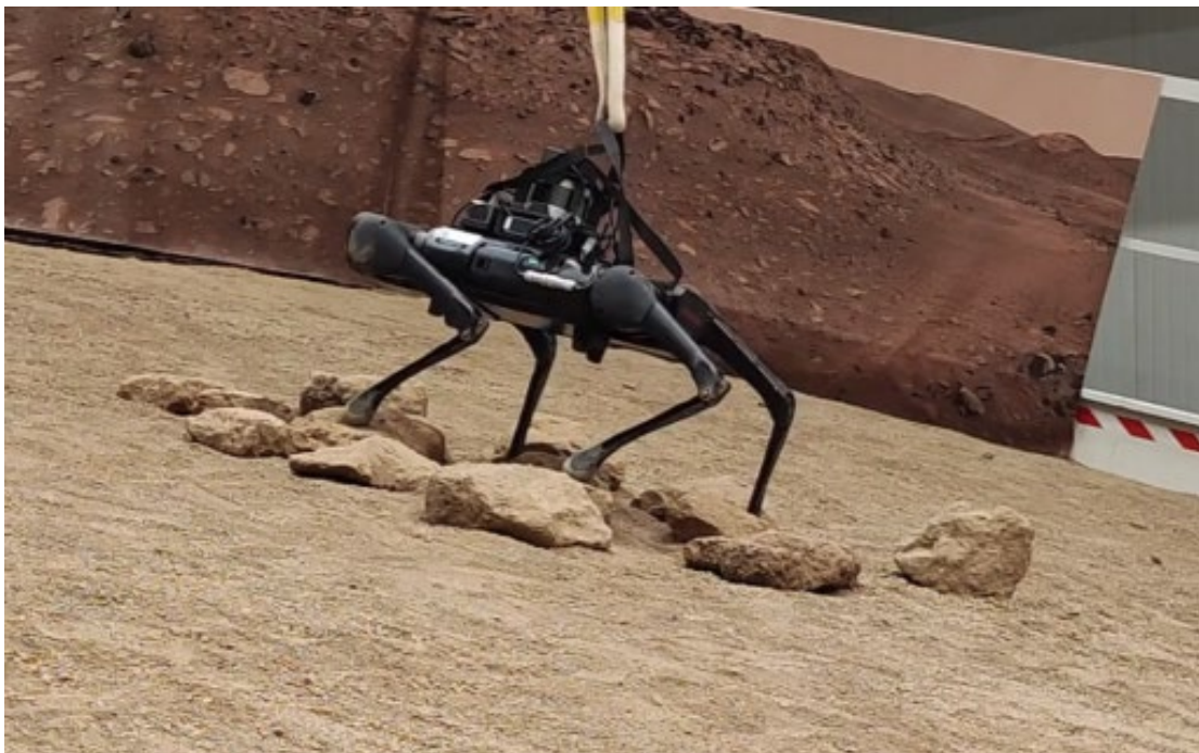
Figure 2: Walking over unconsolidated, unstructured terrain with Aliengo on the tilting platform of ALTEC's Mars Terrain Simulator with rocks
