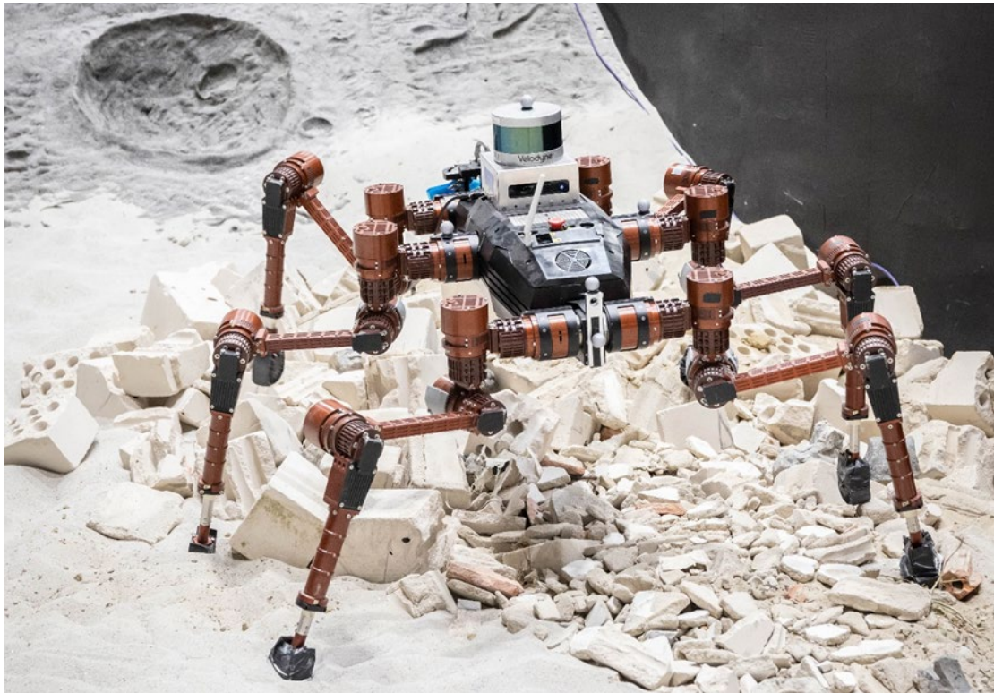
Figure 3. Walking over unconsolidated, unstructured terrain with Crex in DFKI's space exploration hall.
