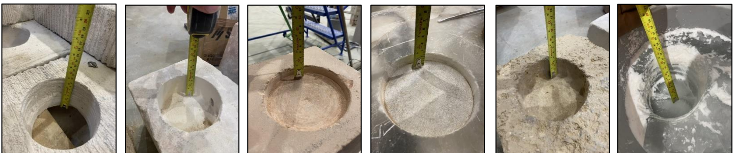
Fig. 2: The results of drill campaigns in aircrete, limestone, sandstone, gypsum, tuff, and ice. A full 'peck' is around 7cm.
