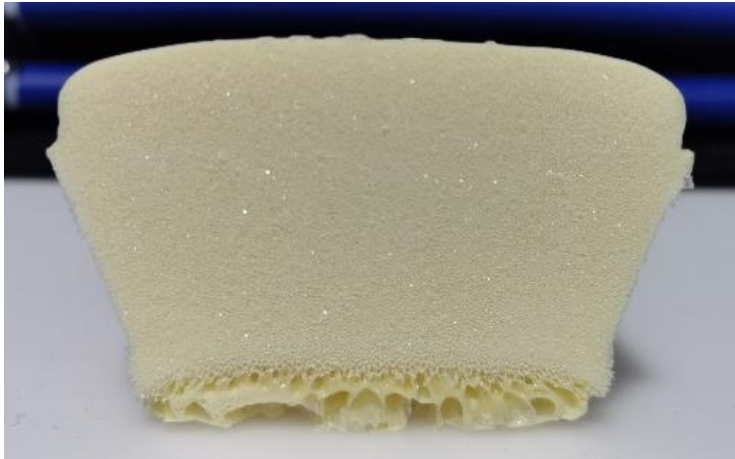
FIGURE 3-1: EXAMPLE OF A PPR FOAM DEFECT – HONEYCOMB
