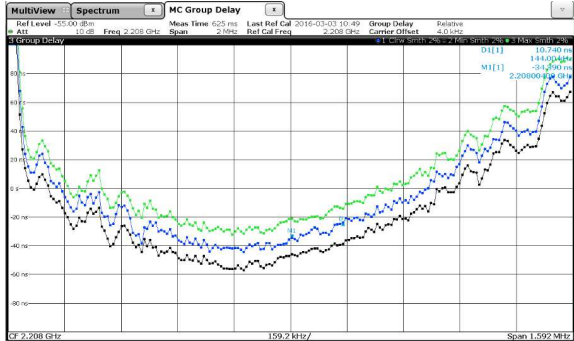
Figure 24 - Group delay variation between 0.3* f_t and 1.7* f_t ( f_t=100 kHz)
