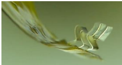
Figure 5-6 – Rodar interconnector after test- (edge bending induced by set-up fixing system)
