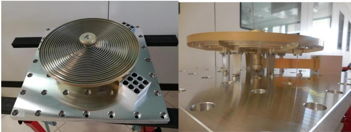
Figure 4.1 Pictures of the DDL antenna prototype.
