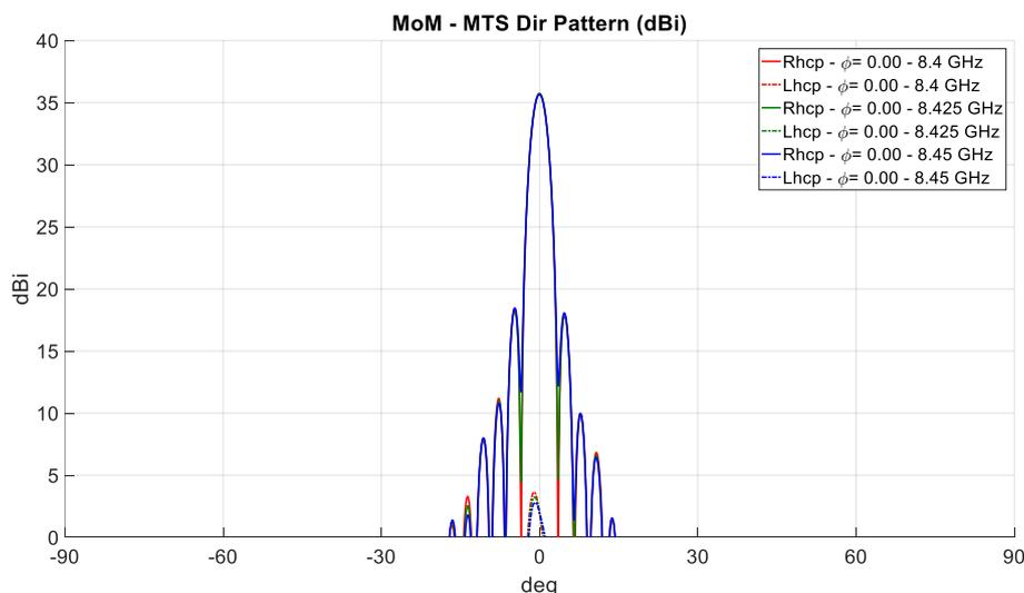
Figure 3.2 Directivity pattern of the Tx MTS antenna at 8.4, 8.425 and 8.450 GHz for the baseline solution. Solid line: co-polar component; dashed line: cross-polar component.
