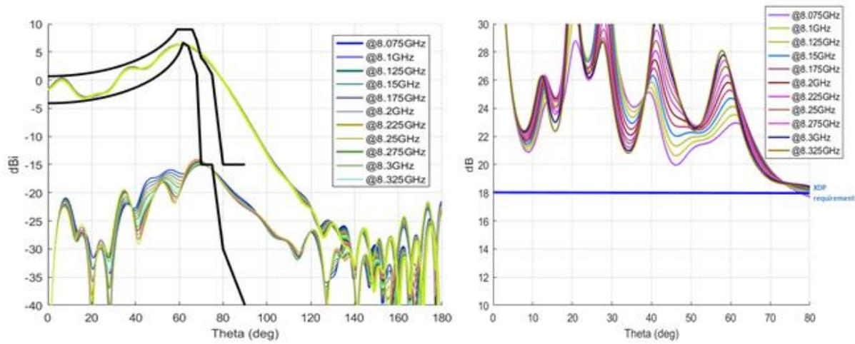
Figure 3.6 Directivity radiation pattern of the optimized grooved-type PDHT antenna (left), XPD variation vs the observation angle theta for various frequencies (right).
