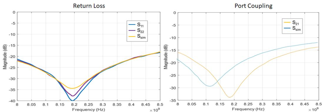
Figure 4.2 Comparison between the measured and simulated scattering parameters at the input ports: return loss (left), port coupling (right).
