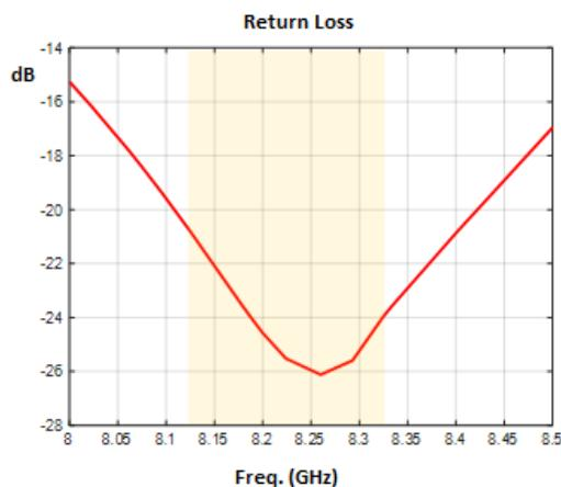
Figure 3.8 Reflection coefficient at the input port of the groove-type PDHT antenna.
