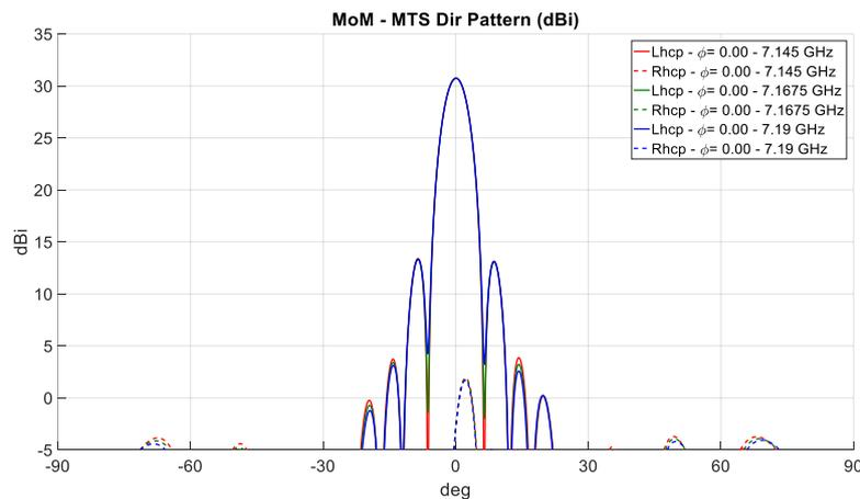
Figure 3.4 Directivity pattern of the Rx MTS antenna at 7.145, 7.1675 and 7.190 GHz along the azimuthal cut at  $\varphi=0$  (spectral line  $\nu=0$ ) for the baseline solution.
