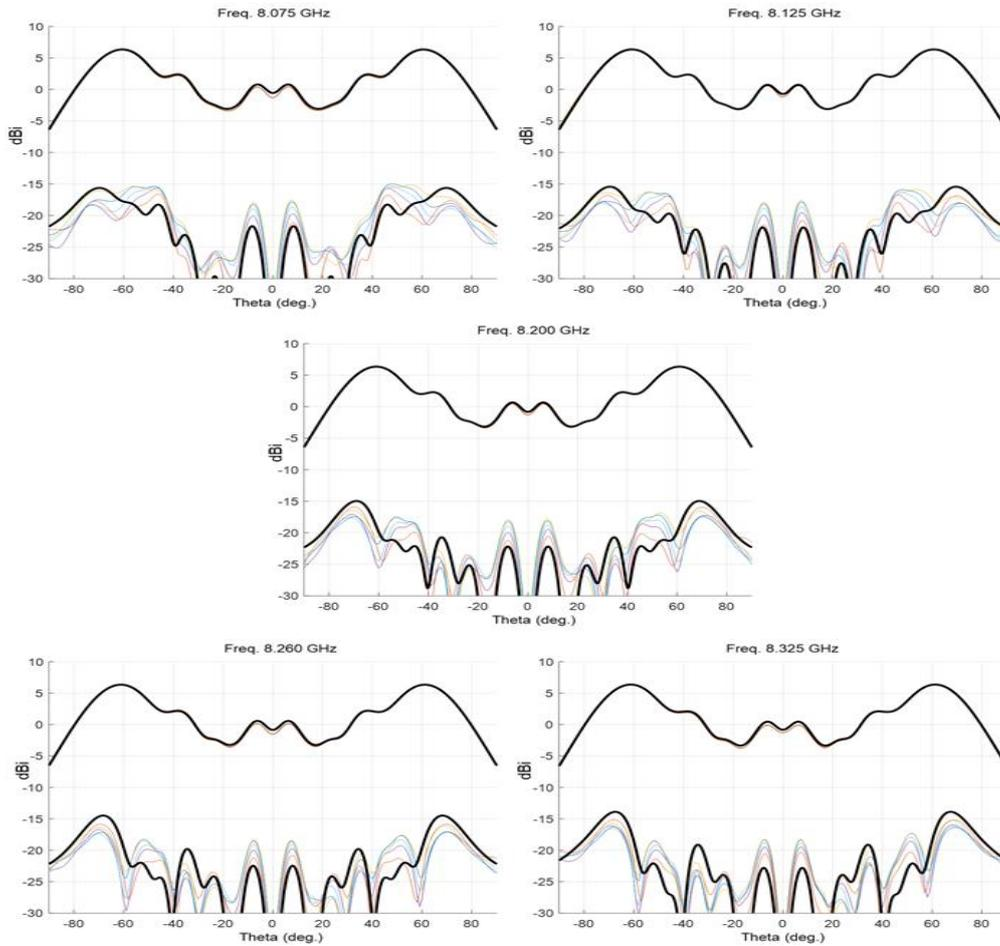
Figure 4.3 Measured gain radiation pattern for various azimuthal cuts for the co and cross polarization at a five frequencies inside the . The black lines are relevant to the predicted radiation pattern.
