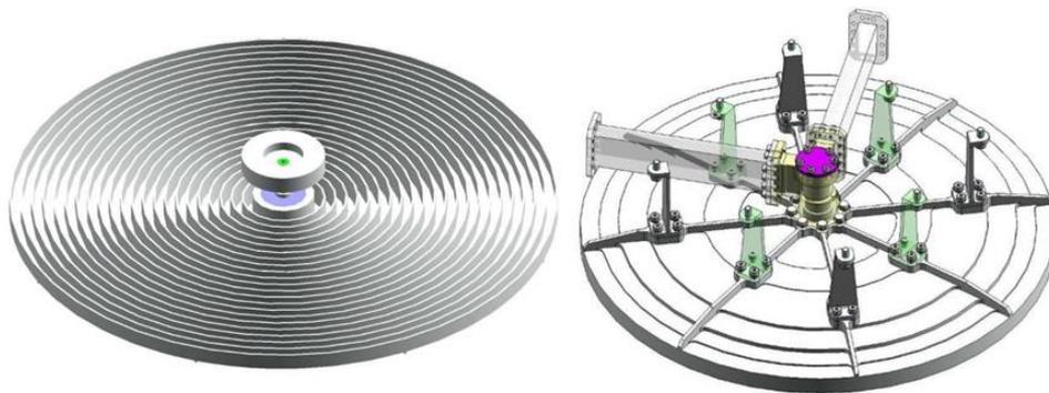
Figure 3.5 Final PDHT antenna configuration.
