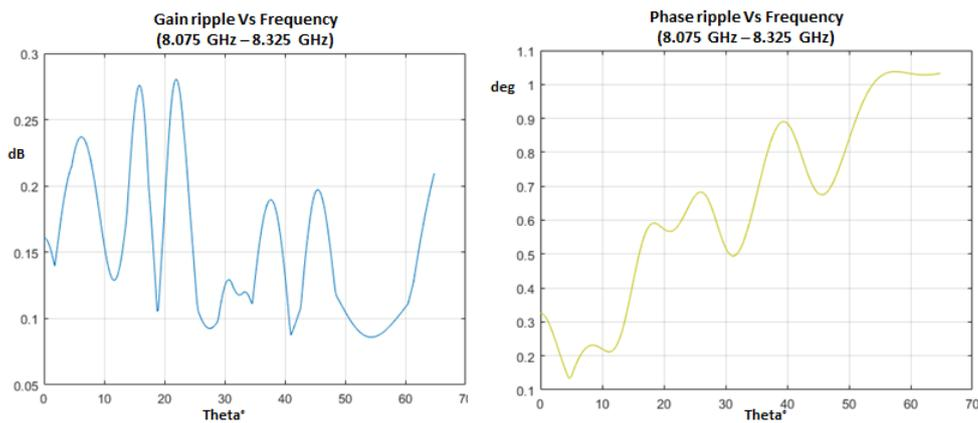
Figure 3.7 Gain ripple Vs Frequency Characteristics (Left), Phase ripple Vs Frequency Characteristics (Right) in the frequency range between 8.075 GHz to 8.325 GHz.
