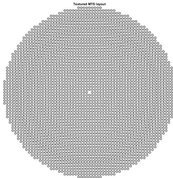
Figure 3.3 Textured layout for the RX antenna
