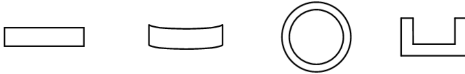
Figure 2 – Candidate Boom profile, Left to right; Flat Bar, Curved Bar, Tube, Channel
