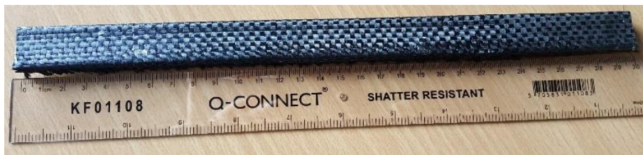
Figure 6 – Section of Pultrudate post manufacture
