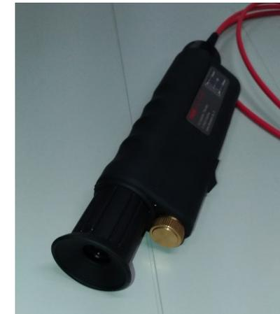
Fibre inspection microscope
