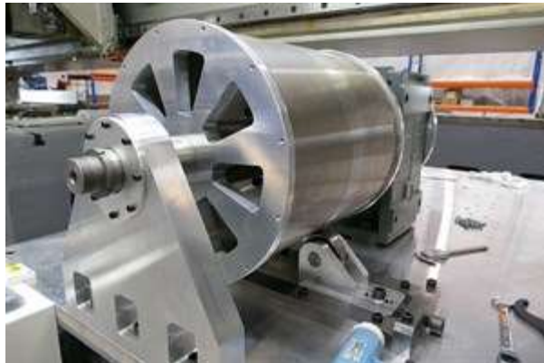
Figure 11 TWI developed tooling to support circumferential FSW trials.
