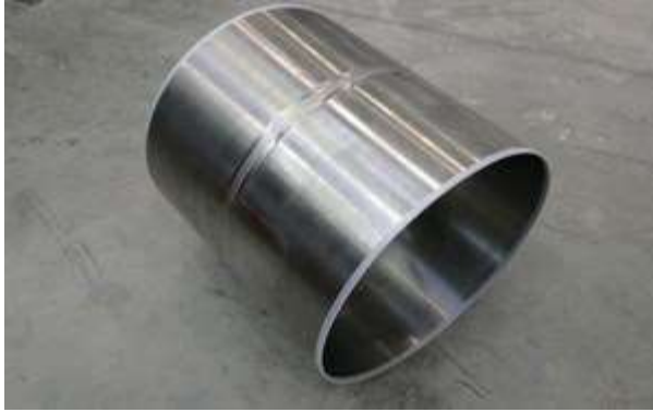
Figure 13 First full circumferential weld.
