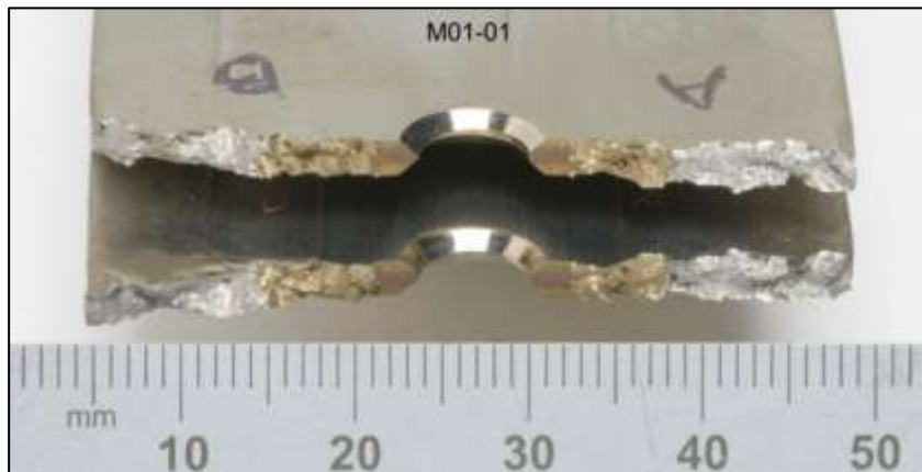
Figure 16 Cast Ti-6Al-4V Alloy FSW - Fracture toughness testing.
