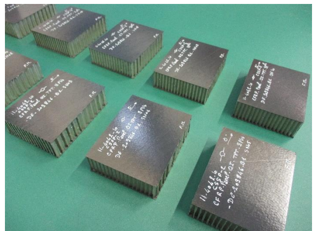
Phase 1 – Edgewise compression test coupons
