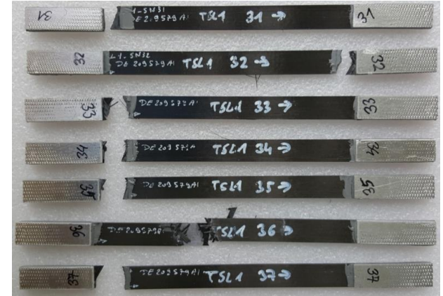
Figure 5: Typical failure modes of tensile test coupons QI TRADI.
