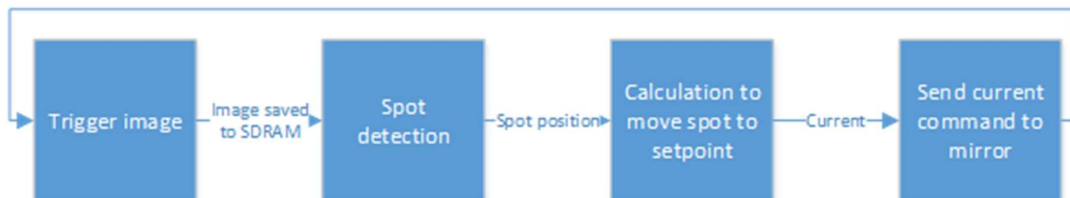
Figure 2: Combined active alignment system algorithm block diagram.
