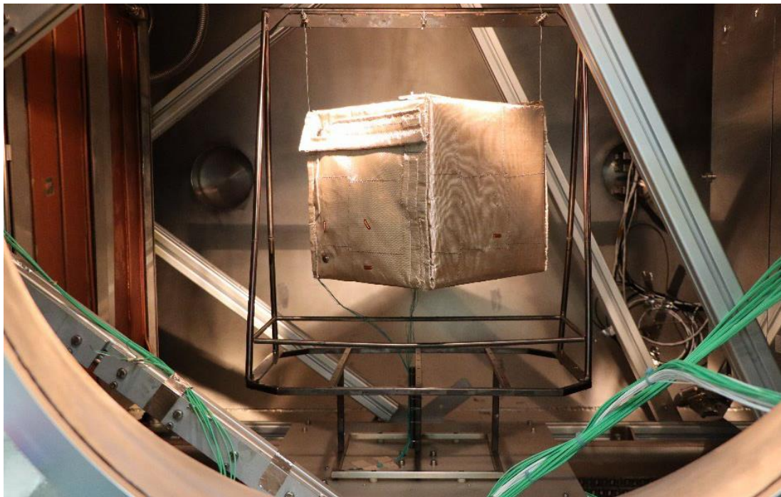
Figure 6-3: Aerobraking MLI Cube in the FTV chamber for thermal cycling
