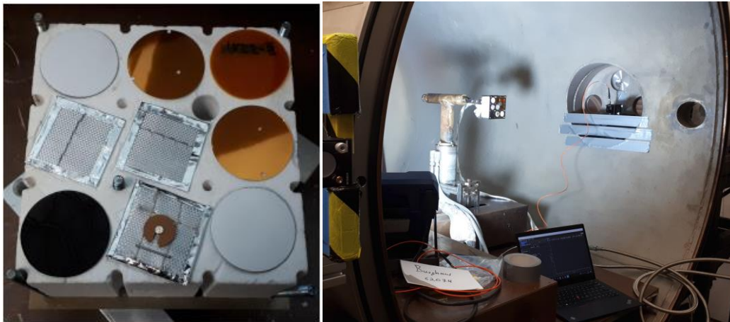
Figure 5-1: Samples for the test and sample holder in the plasma wind tunnel chamber
