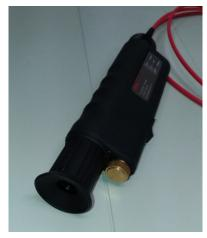
Fibre inspection microscope
