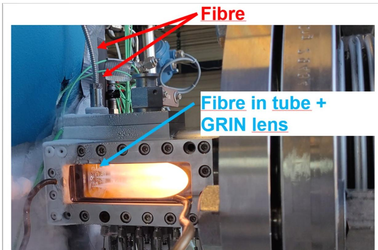
Figure 1: successful ignition for the test configuration “FU2-LAI-GRIN” of the CCN1-test campaign
