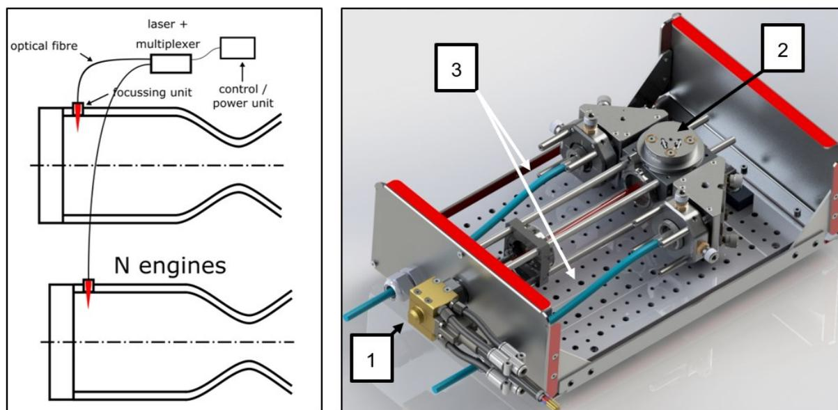
Figure 1: Concept and CAD of the laser (1), multiplexer (2) and optical fibres (3) of the fibre-based laser ignition system
