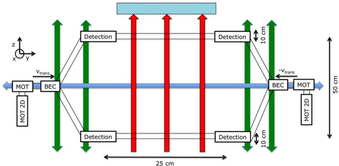
**Figure 1:** Schematic of the concept proposed for the implementation of a spaceborne Gravity Gradiometer based on laser-cooled atom interferometry. The sections at both ends (labelled MOT2D-MOT-BEC) would be the ultracold atom source, and the area in the centre (between and containing the detection areas) would be the atom interferometry chamber (extracted from RD01)
