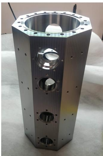
**Figure 3:** Photograph of the main chamber body
