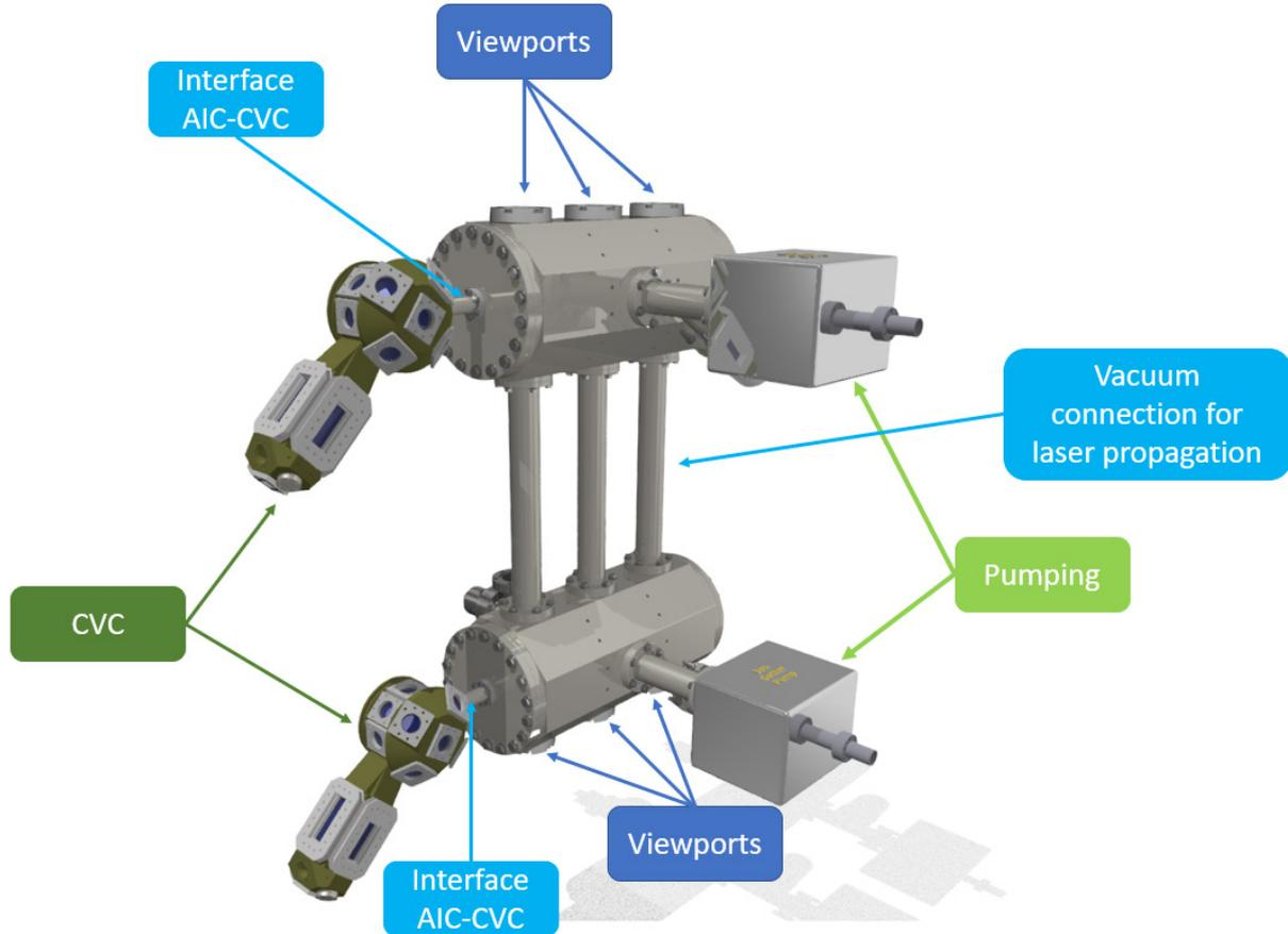
**Figure 2:** Conceptual design of the AIC. Labelled are the key features.
