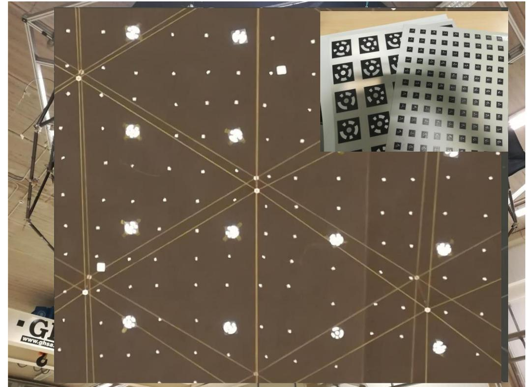
Final LDR setup with film retroreflector targets and absorbing sheet
