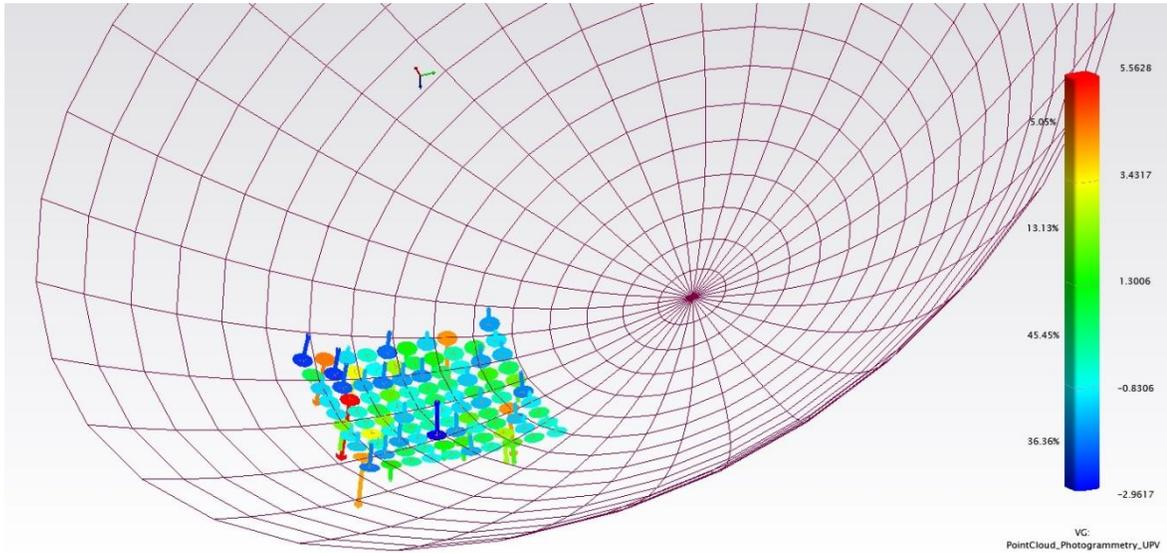
**Paraboloid best-fit to photogrammetry point cloud**
