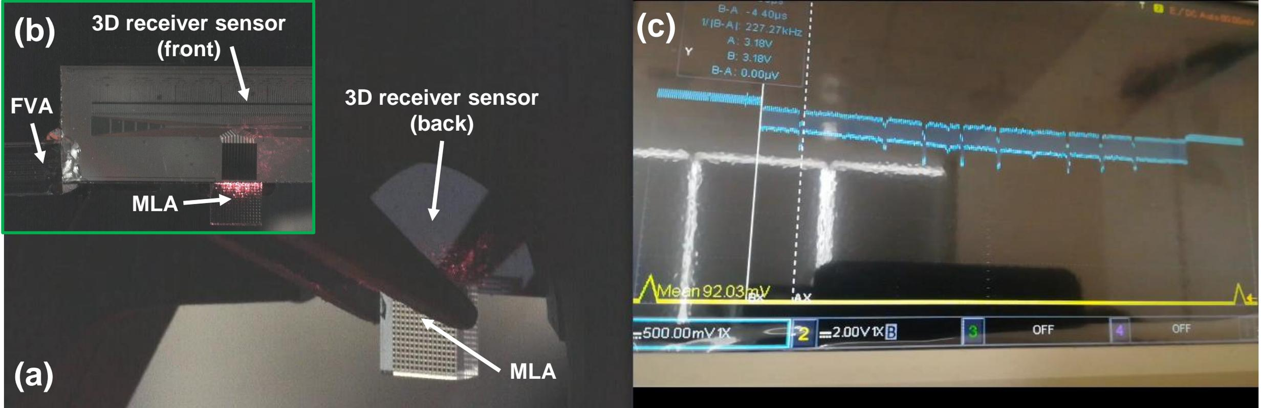
Microlens array alignment. (a) Back view; (b) Front view
