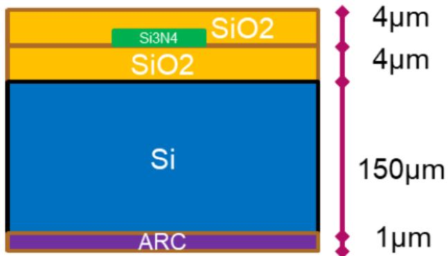
3D receiver sensor – stack of layers
