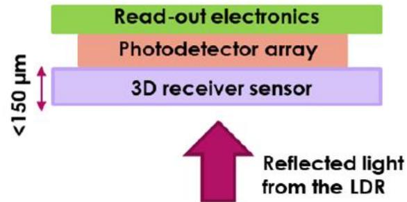
3D receiver sensor – light coupling from the back-side using gratings
