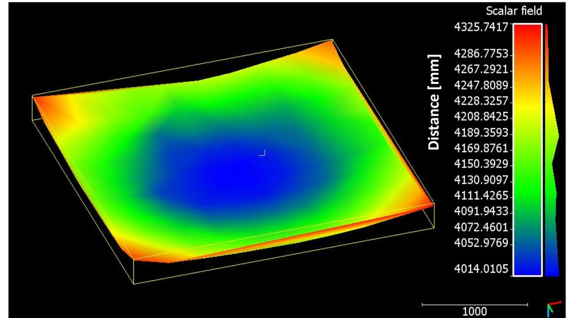
Point cloud obtained with the metrology breadboard and Surface reconstruction
