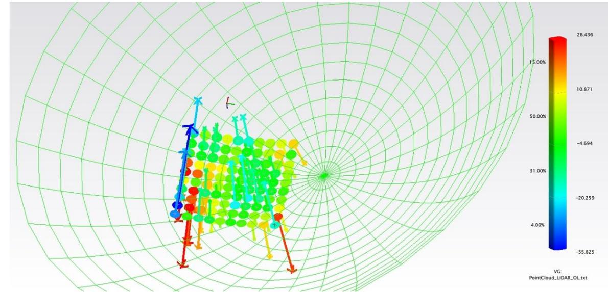
**Best fit of breadboard point cloud to previous paraboloid**
