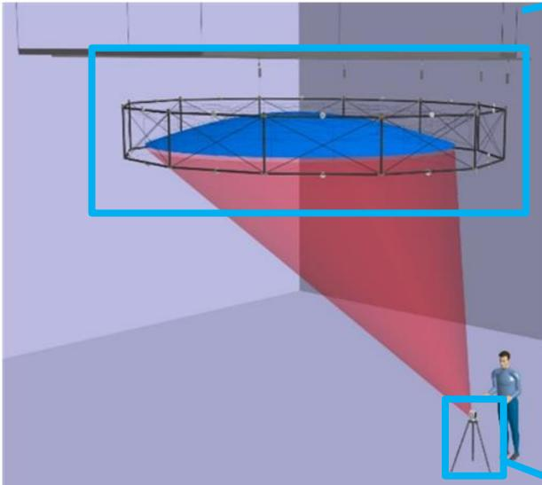
**Goal: Metrology system at TRL 4 - 10  $\mu\text{m}$  accuracy @ 10 m for large diameter LDRs**
