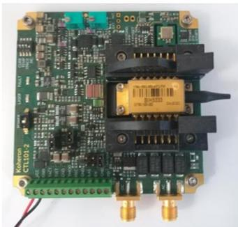
Low noise continuous wave laser at 1550nm
