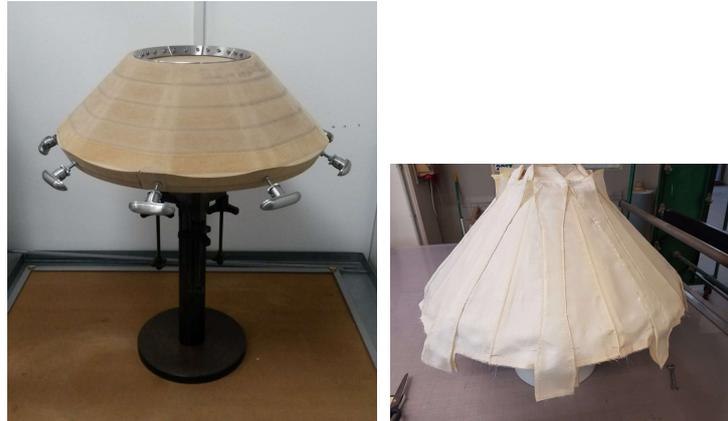
Figure 8 - The Sewing frame and the process of manufacturing the flexible TPS
