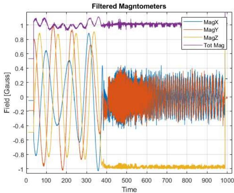
Figure 7 – Magnetometer of Z axis showing stable attitude across the re-entry
