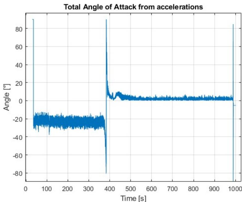
Figure 6 – Angle of Attack of the Capsule calculated from the accelerations
