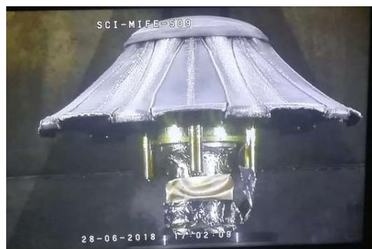
Figure 11. Details of the TPS parts after the SCIROCCO test completion
