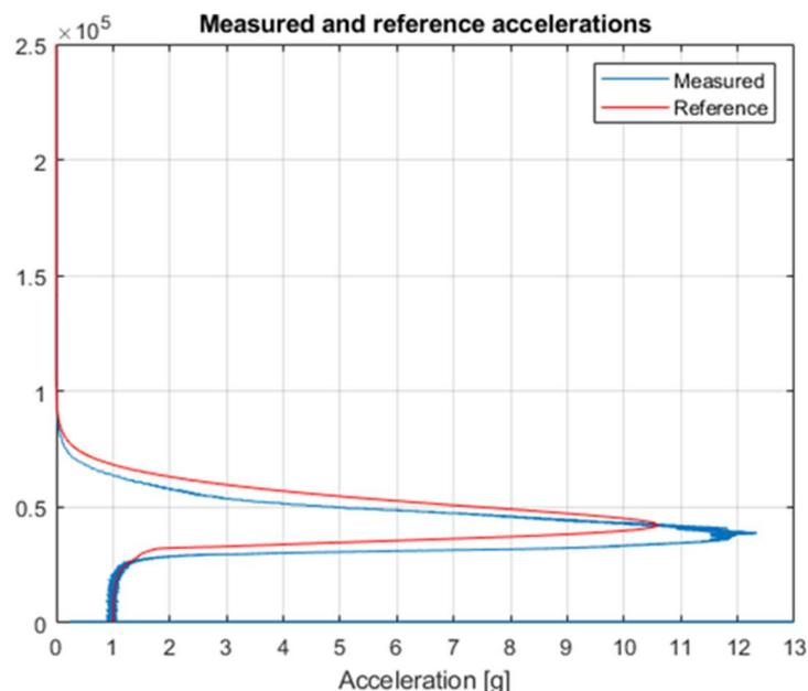
Figure 5 Comparison of flight and predicted load factor during the re-entry
