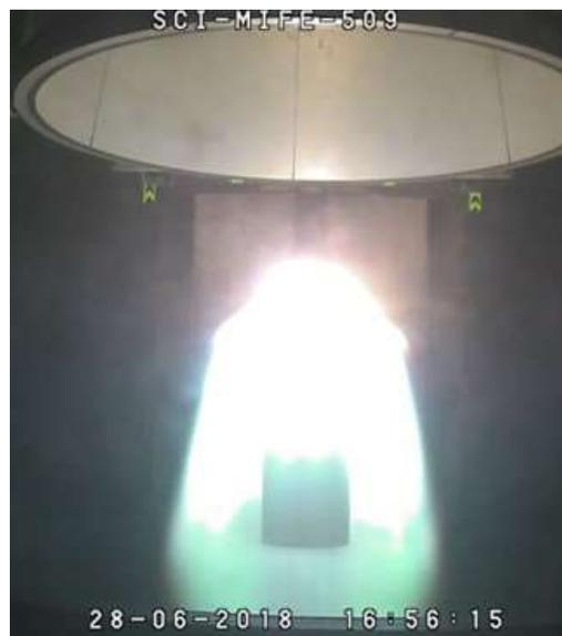
Figure 10. The GD in the SCIROCCO plasma flow
