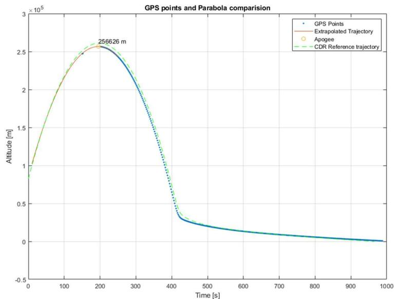
Figure 3 Altitude vs time. GPS data, extrapolated trajectory, apogee and reference trajectory.
