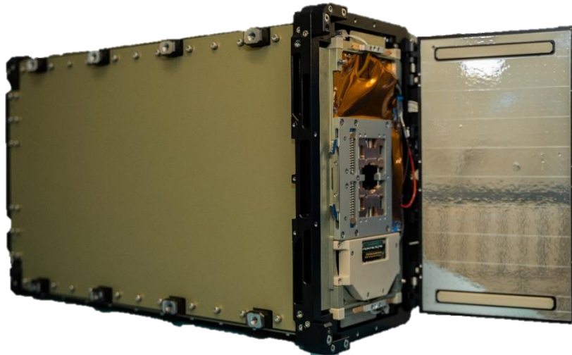
Figure 10: Flight Model of Deep Space Deployer.
