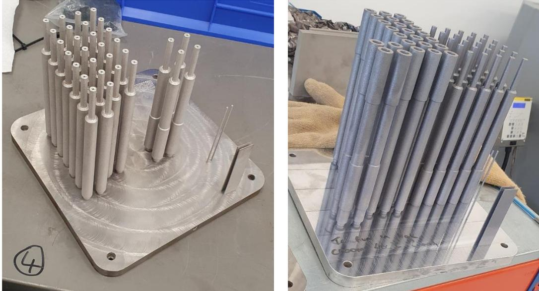
*Figure 1: ALM thermosyphon samples after metal 3d-printing.
