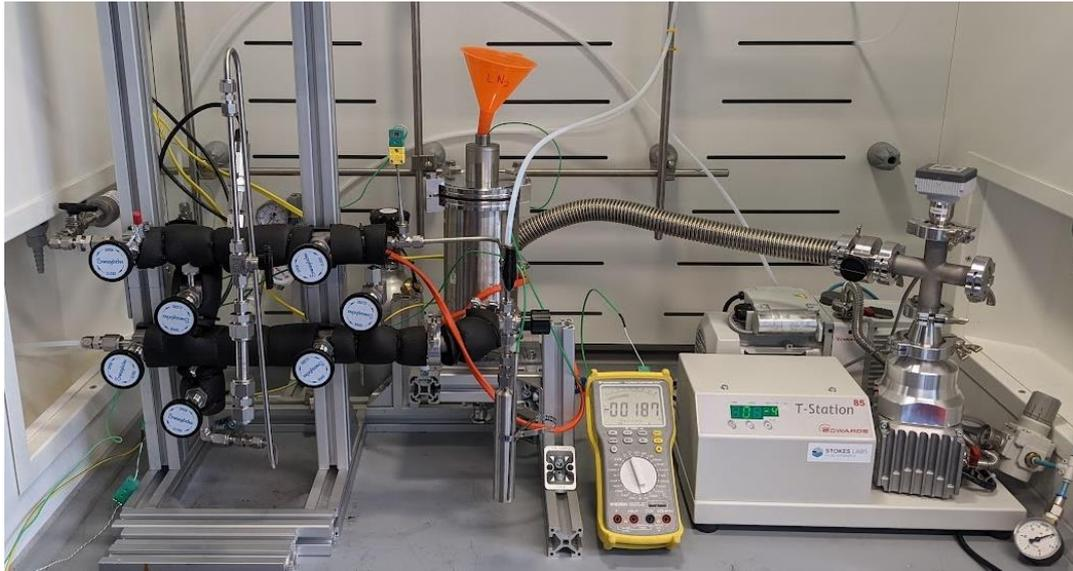
*Figure 2: Gas working fluid filling test bench*
