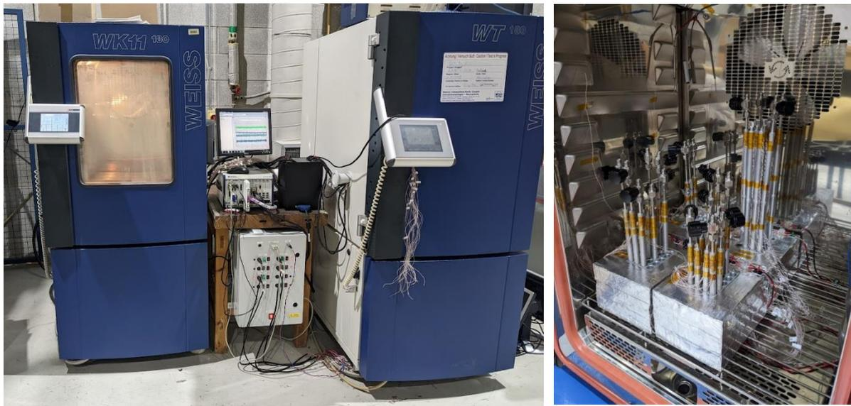
*Figure 3: Environmental Chambers. Left: Exterior with controller and data logging equipment. Right: chamber interior with samples mounted in heater blocks*
