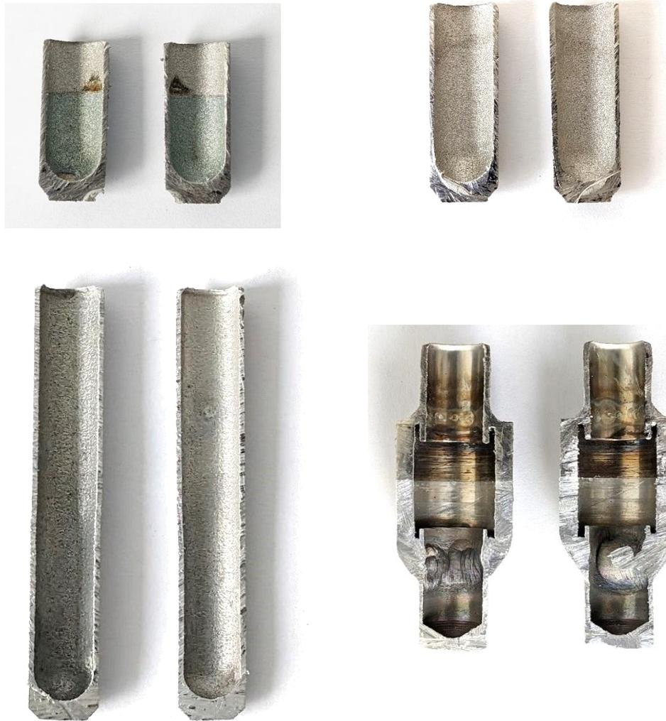
Figure 6: Cross - sectioned samples. Top right: SS316L ALM-water. Top left: SS316L-ammonia. Bottom left: AlSi7Mg-ammonia, Bottom right: Bimetal-toluene
