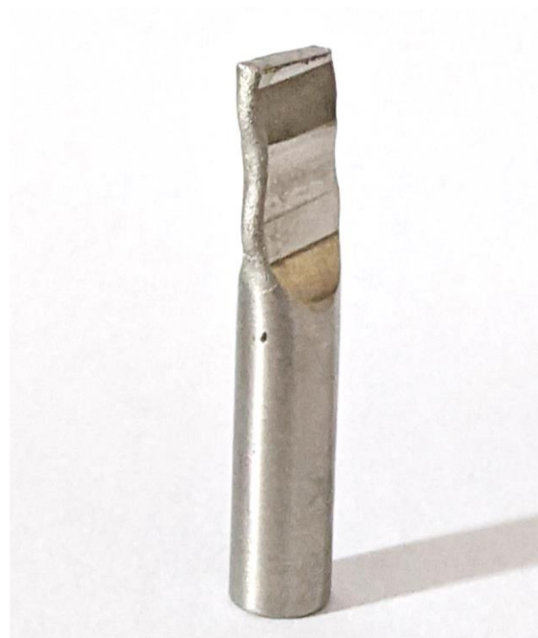
SS316L (6.35 mm OD, 2.0 mm ID) 6.35 mm crimp
