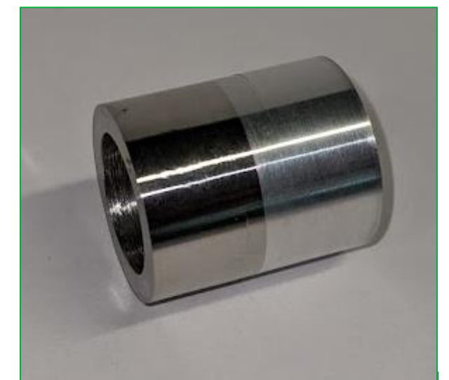
Spur Industries, Inc. roll bonded Al3003-SS304L bi-metallic junction.
