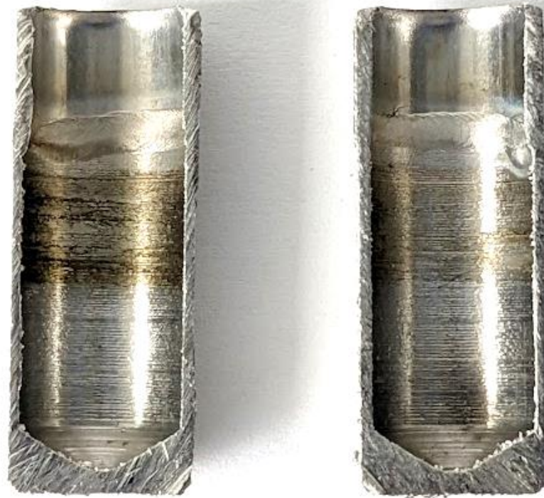
SS316L conv. Brown corrosion in L.-V. interface region
