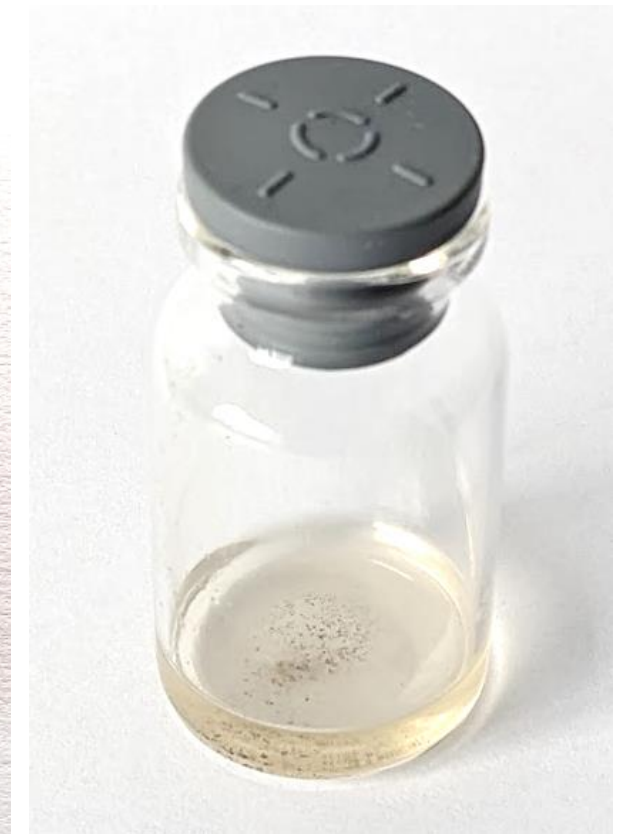
Water Orange tint and contained some loose particles.
