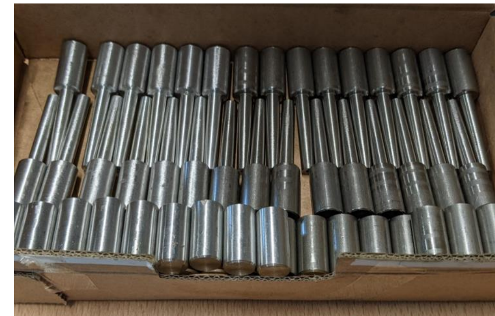
Al6061 and SS316L end caps and filling tubes
