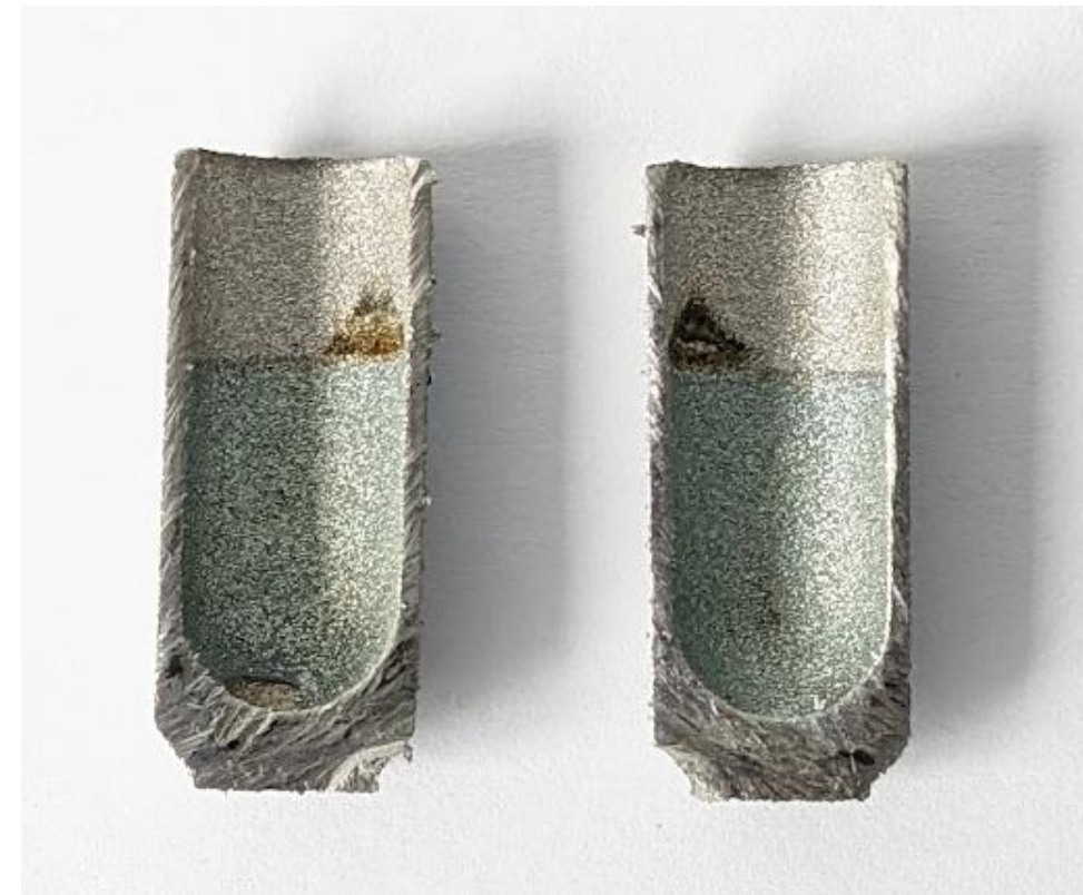
SS316L ALM Light green colour in liquid region. Orange colour in L.V. region.
