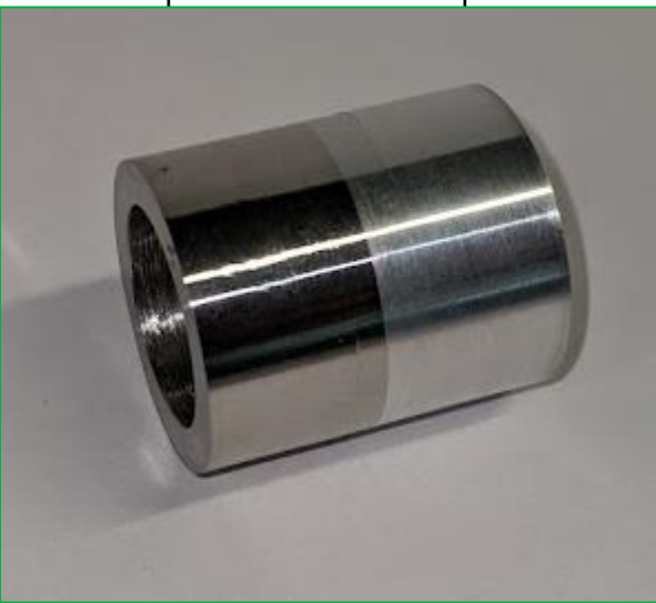
Spur Industries, Inc. roll bonded 3003 Al – 304L SS bi-metallic junction.
