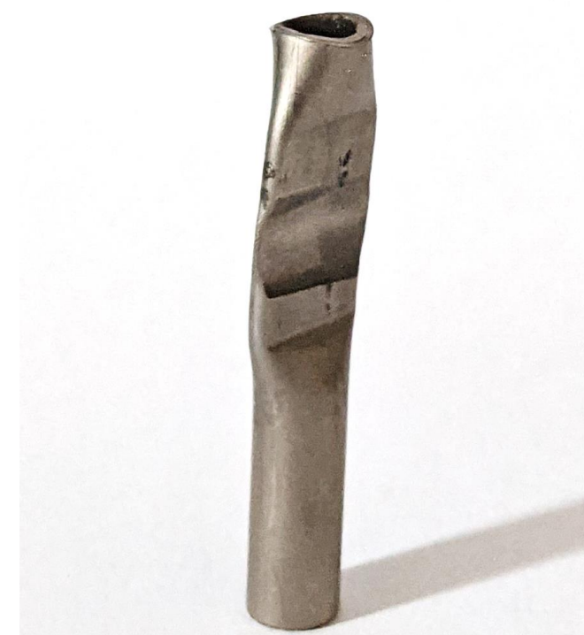
Ti CP Grade 2 (6.35 mm OD, 4.55 ID) 12.7 + 6.35 mm crimp Failed He leak test
