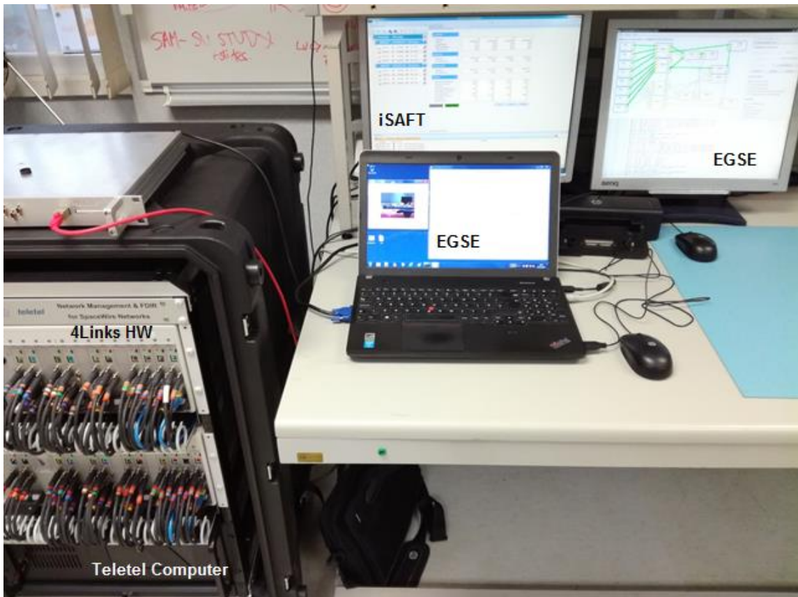
Figure 9: N-MaSS Demonstrator (HW racks, EGSE and iSAFT)
