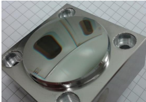
Figure 3 : left : Picture of the machined free form grating - right : microscope view of grating groove
