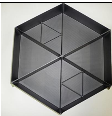
JWST M1 segment : mockup definition (0,5m)
