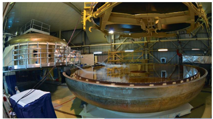
Figure 3-7: Illustration of the technologies available in observatories: (Left) Joule effect Evaporation chamber - Calar Alto (Right) Magnetron sputtering Vessel - Gemini South
