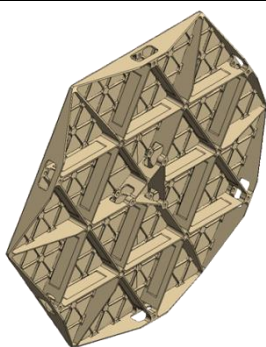
JWST M1 segment : mockup definition (0,5m)
