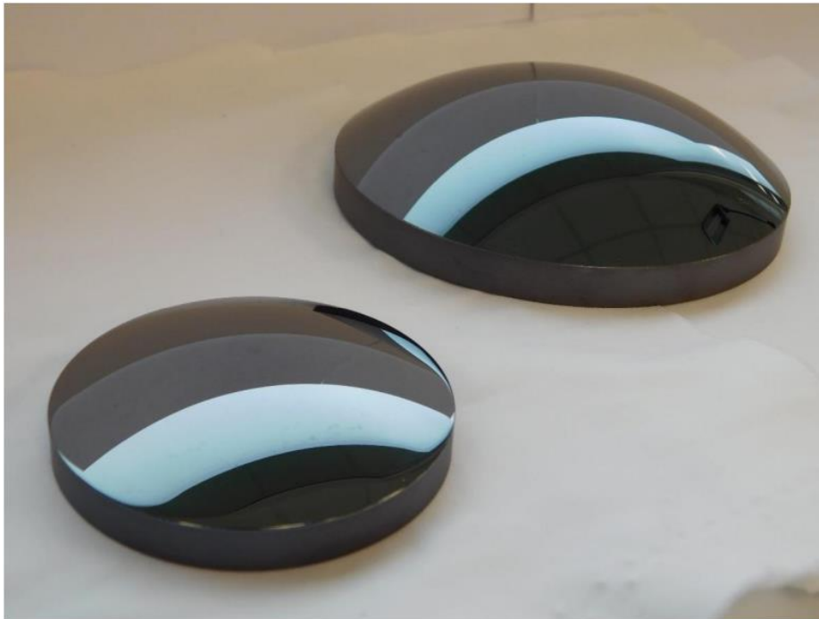
Figure 5 Aspherical lenses made of IG2
